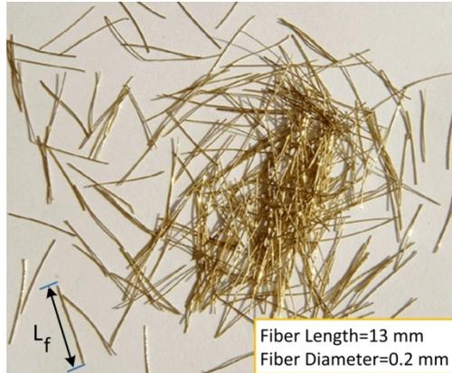
Figure 3-1: Short steel fibers,  $l_f=13$  mm and  $d_f=0.2$  mm.
