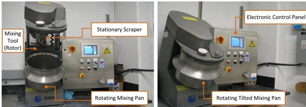
Figure 3-2: High performance mixer with inclined pan.
