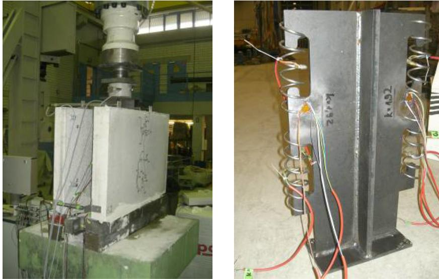
Figure 2-36: Push-off test with puzzle-strip shear key and spiral springs (Abramski et al. 2010).
