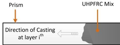
Figure 3-7: Top view of casting method.
