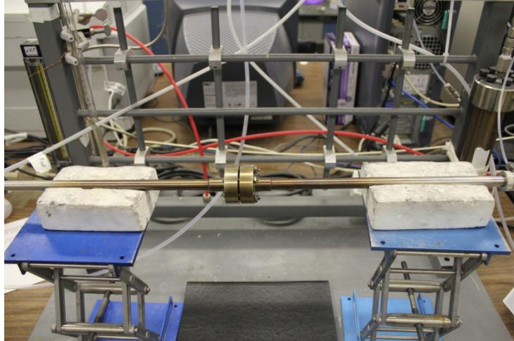
Figure 3.5 Flanged membrane chamber for permeation test
