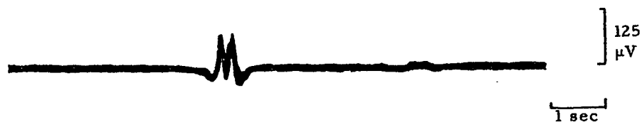
Figure 19. Detached antennal preparation. Response to benzene vapour delivered by the bubble apparatus. Allowing for the greater scale of this recording compared with that of figures 16, 17 and 18, this response is similar to that produced by insect repellents.
