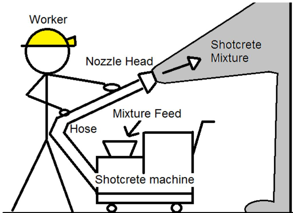
Figure 2.1. Typical shotcreting process
