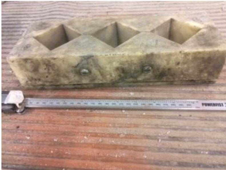
Figure 4.4. Mold used to create cubic samples
