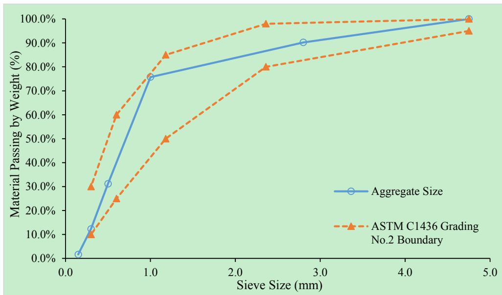
Figure 4.2. Sieve analysis result for the aggregate utilized in this research
