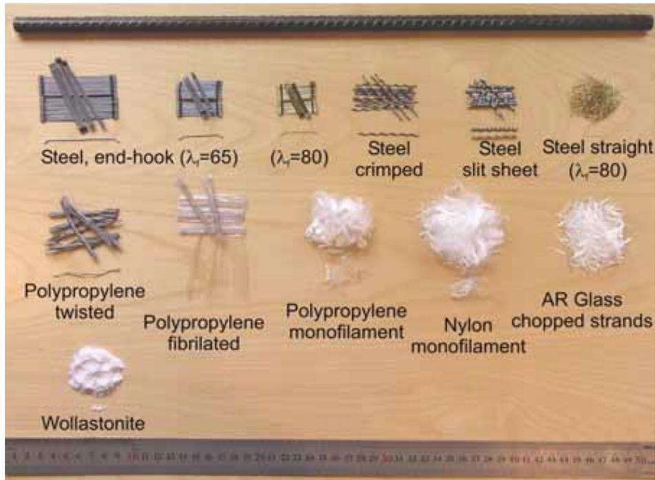
Figure 2.5. Examples of fibers commonly added to concrete (Löfgren, 2005), available under Berlin Declaration on Open Access to Knowledge in the Sciences and Humanities
