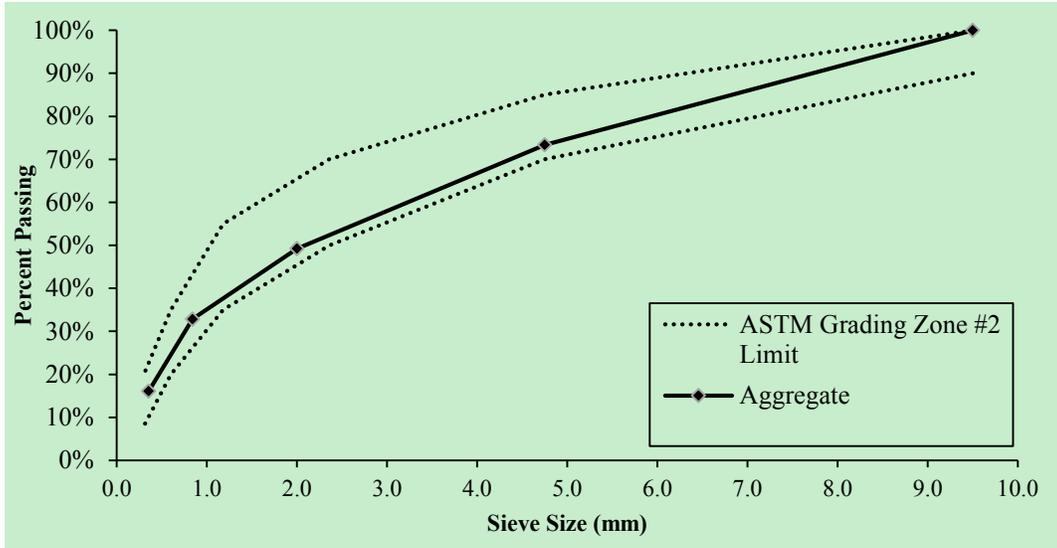
Figure 3.2. Aggregate size distribution and grading limit
