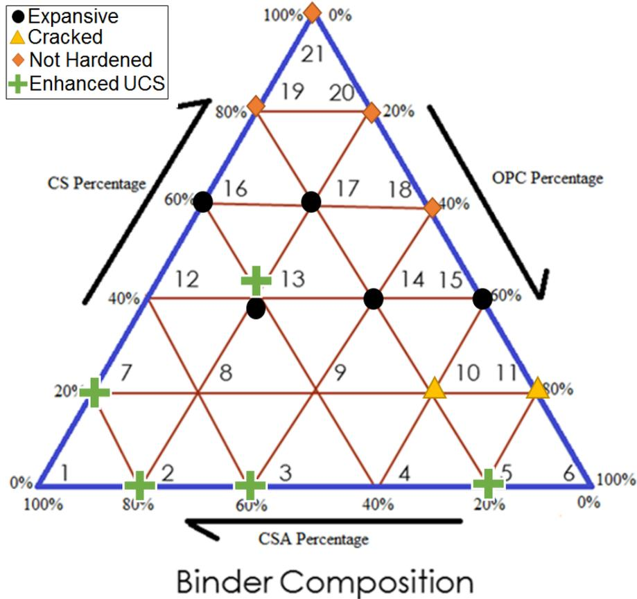
Figure 3.11. Preliminary CSA-OPC-CS Shotcrete Mixture Classification
