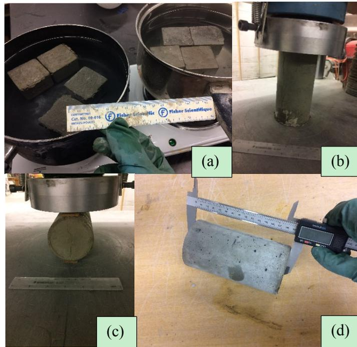
Figure 4.6. Tests performed on the samples: (a) boiling of cube samples for density, absorption, and voids determination; (b) compression of mixture sample; (c) STS determination using a loading machine; (d) measurement of dimension of the sample
