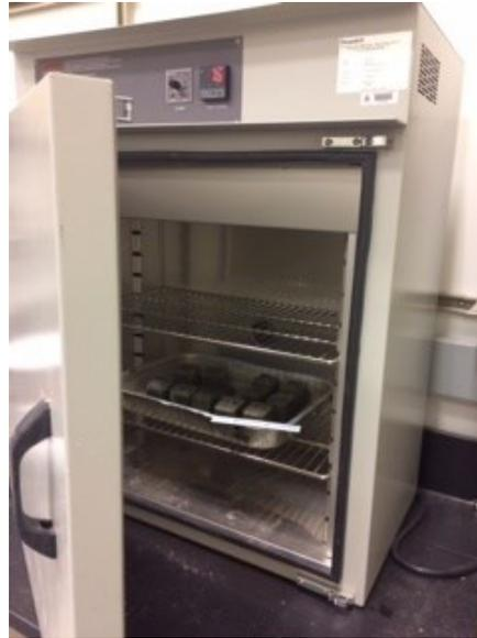
Figure 4.5. Oven used for the drying of the samples
