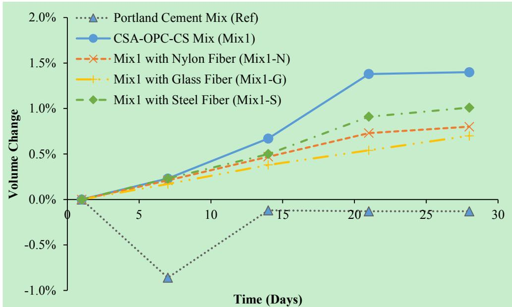
Figure 4.7. Volume changes of mixtures with various fibers over time
