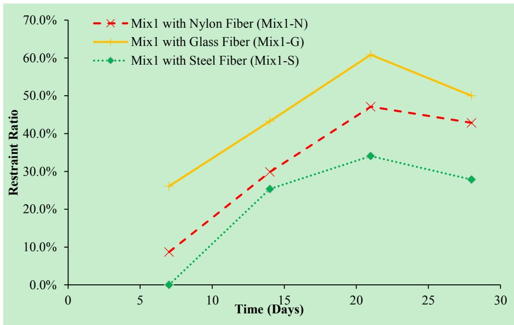
Figure 4.8. Restraint ratio of fiber-reinforced CSA-OPC-CS mixtures over time
