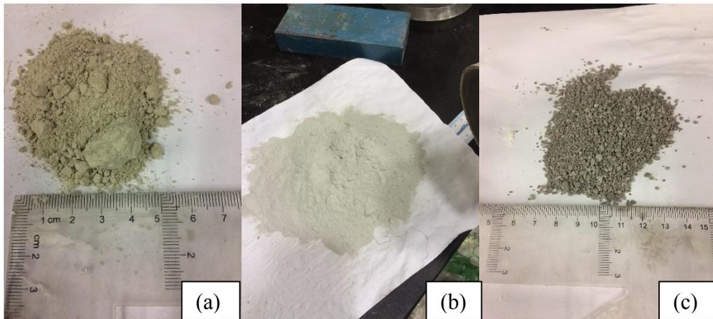
Figure 3.1. Binder materials used in this research: (a) CSA; (b) OPC; and (c) CS
