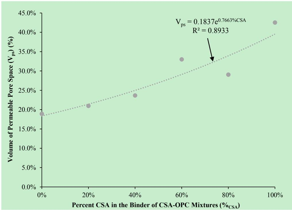
Figure 3.7. Effect of utilizing CSA over OPC on volume of permeable space
