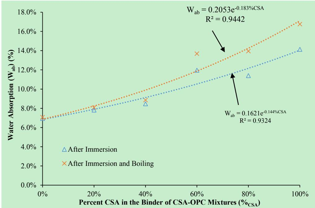
Figure 3.6. Effect of utilizing CSA over OPC on water absorption
