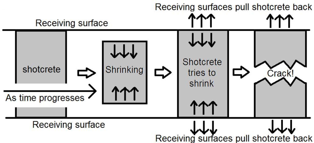
Figure 2.3. Shrinkage cracking mechanism of shotcrete
