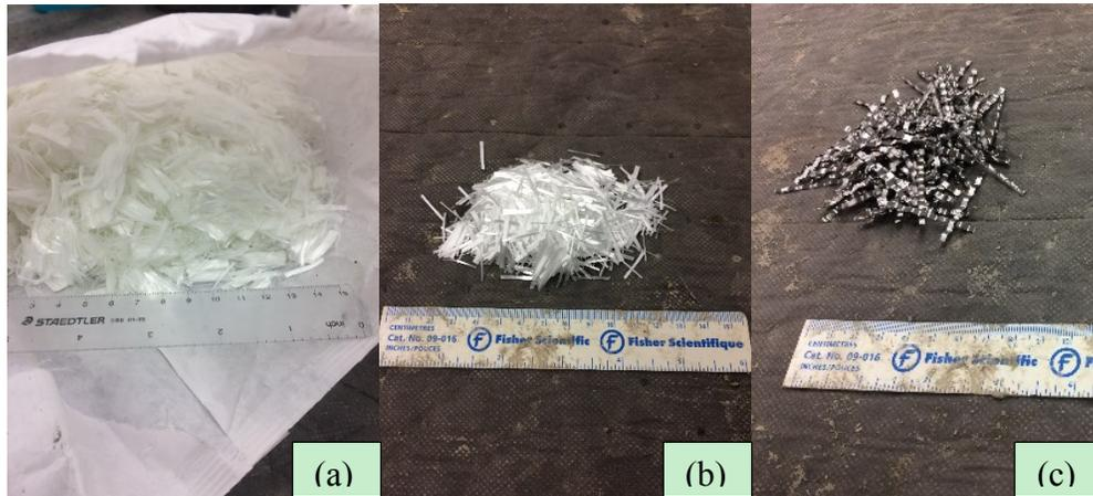
Figure 4.3. Various fibers utilized in the research: (a) nylon fibers; (b) glass fibers; (c) steel fibers
