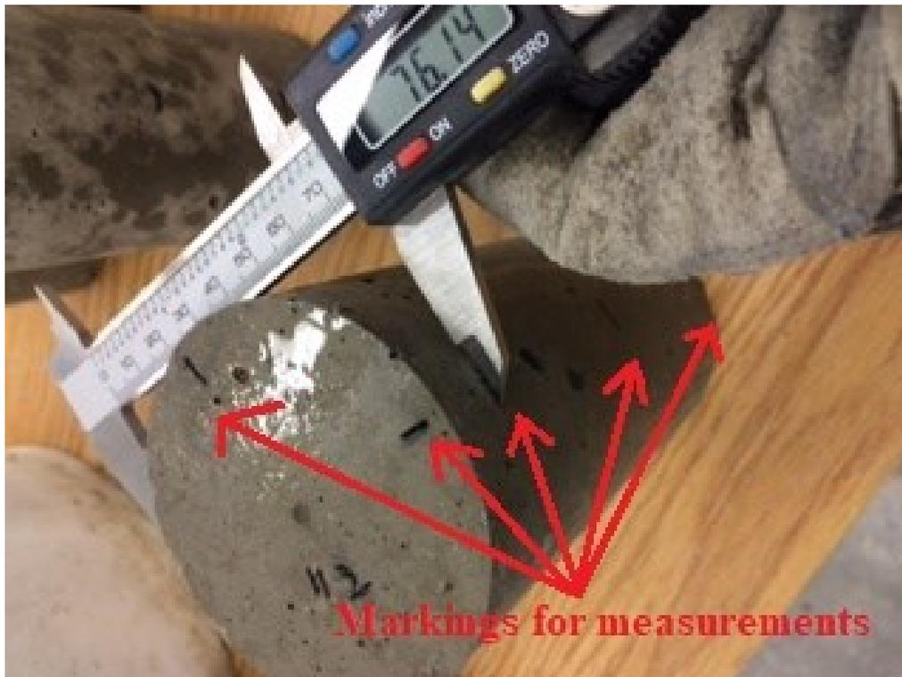
Figure 3.5. Volumetric measurements on cylindrical samples
