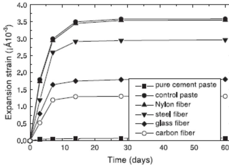
Figure 2.6. Effect of different types of fibers on restraint of paste expansion (Chen & Liu, 2003), figure usage permission granted by Elsevier
