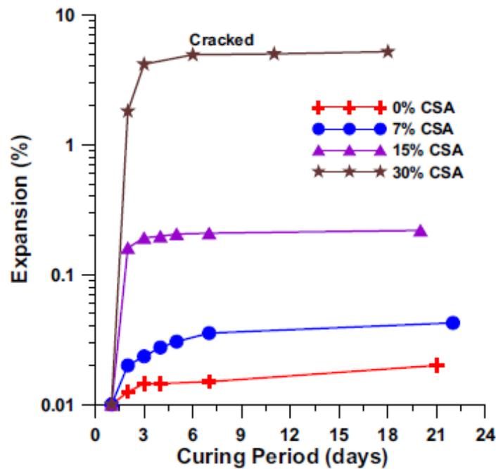
Figure 2.4. Expansion of OPC-CSA blends (Chaunsali et al., 2015), figure usage permission granted by John Wiley and Sons
