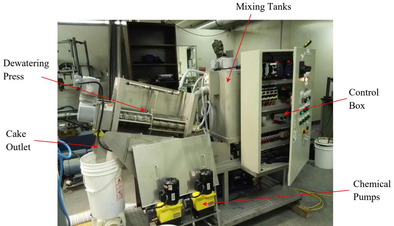
**Figure 2.1.** Front view of the volute screw press.
