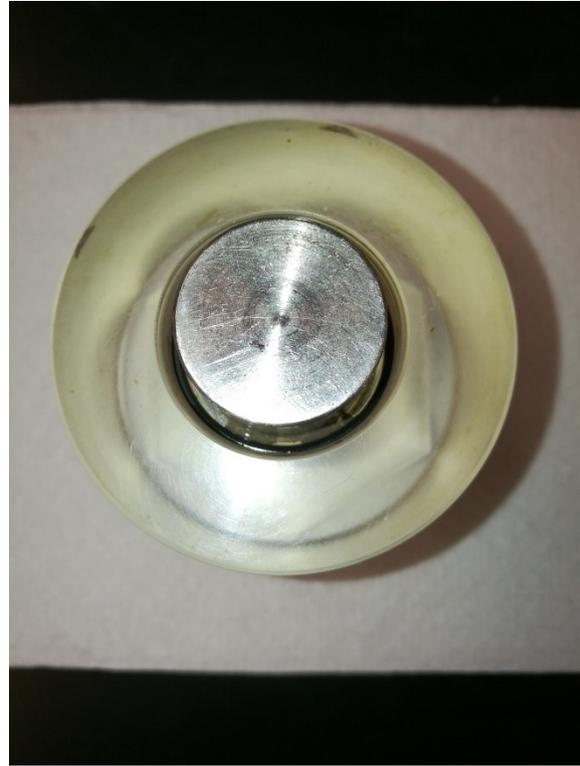
**Figure 5.5.** Third plasticity event characterization for case A300-C1000. Left: an additional CVST stress-strain curve for A300-C1000, indicating an unknown plasticity event at higher response stress. Right: top-down view of the sample chamber effluent trap for this experiment. After liquid removal, small amount of solid sediment was visible. This plateau indicated the onset of a rupture event.
