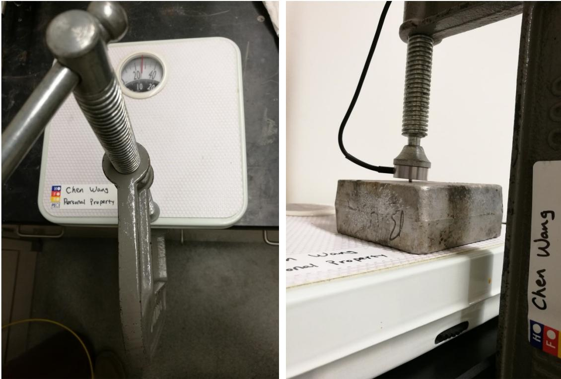
**Figure 3.5.** Force sensor calibration setup. Left: methods of force generation and measurement. Right: close-up view of the sensor and the protective aluminum block during calibration.
