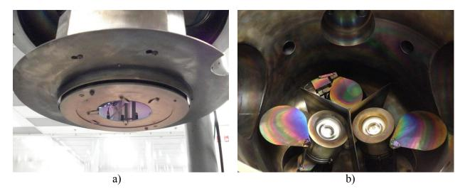
Figure 4-9: a) Loading the silicon substrate. b) Loading the Aluminum targets.
