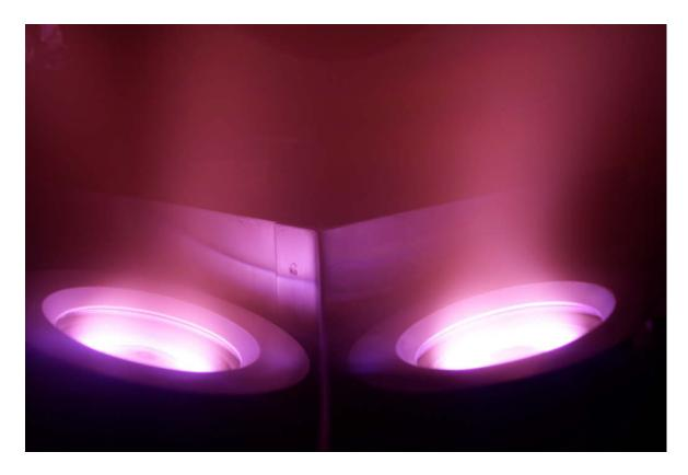
Figure 4-10: Argon/Nitrogen plasma during Aluminum Nitride deposition
