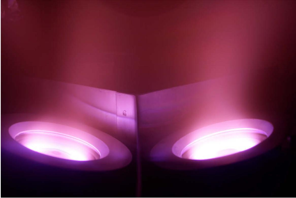
**Figure 4-10: Argon/Nitrogen plasma during Aluminum Nitride deposition**
