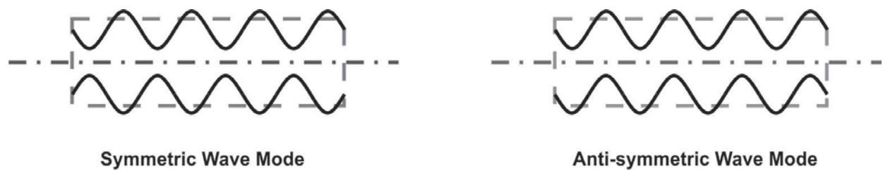
**Figure 2-2: Symmetric and antisymmetric lamb wave modes**
