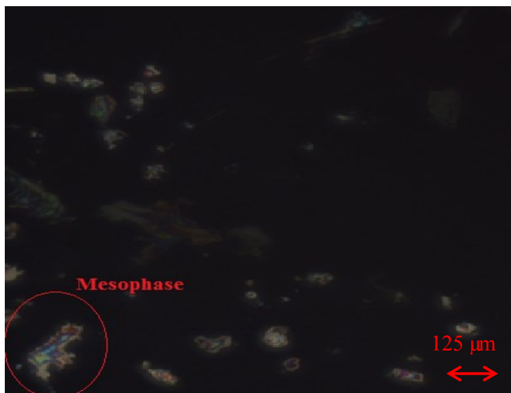
Figure 5-5: Mesophase formation at 200 minutes during pyrolysis when pyrolysis liquids were observed under cross polarized light (200X magnification)
