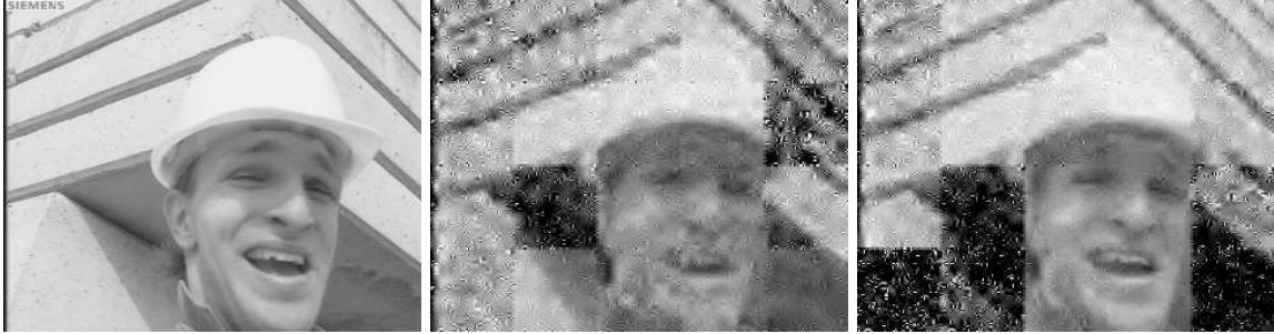
Figure 4.3: Severe undersampling with different sensor modes. Left: original frame 16 of ‘foreman’. Middle: reconstructed frame with all texture-focused sensors and a sampling ratio of 12%; PSNR = 13.7 dB, SSIM = 0.327. Right: reconstructed frame with all motion-focused sensors and a sampling ratio of 12%; PSNR = 11.4 dB, SSIM = 0.375. At this point in the video, the foreman is moving his head toward the upper right corner and there is a slight upward global camera motion.
