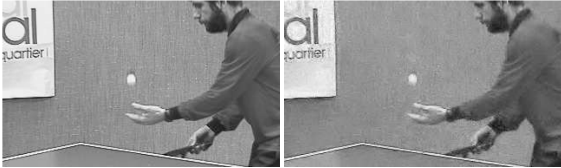
Figure 4.9: Original vs. reconstructed frame 53 of ‘tennis’. PSNR = 28.5 dB, SSIM = 0.738. The quality is uniform throughout all blocks and the sampling ratio is adequate.
