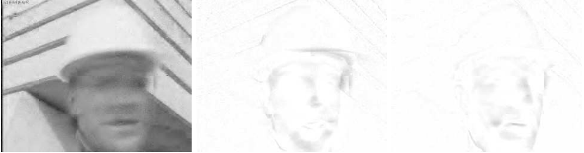
Figure 4.2: An implicit reference frame and two innovation frames. The innovation frames have been luminance-inverted to show detail. The innovation frames are very sparse; the implicit reference frame resembles an average of all frames in the frame group. Note that each block in the implicit reference frame was reconstructed independently using different frame group sizes.
