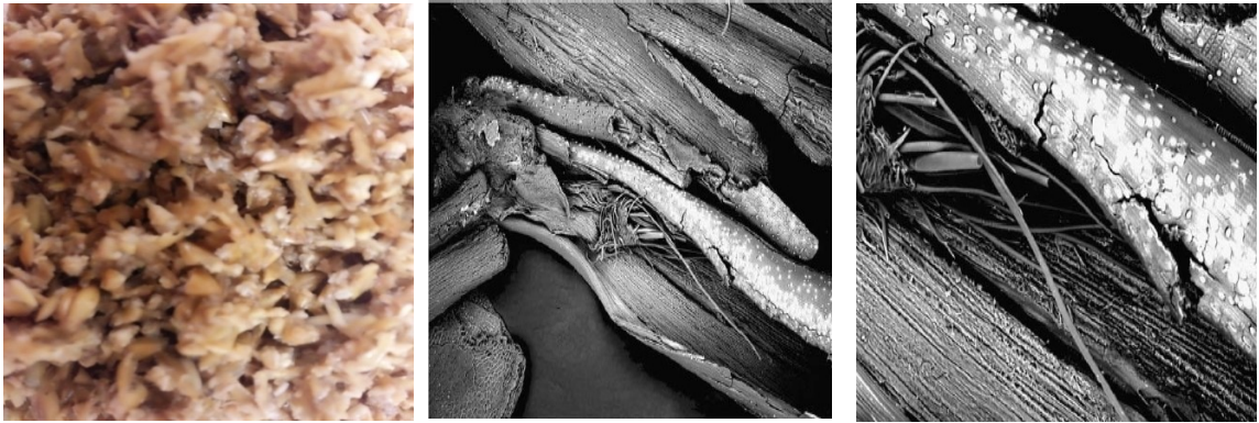
Figure 1.3. (A) Visual (B) Scanning electron microscopic (x100) (C) Scanning electron microscopic (x300) appearance of BSG (Scanning electron microscopic images adapted from Mussatto et al., 2006).
