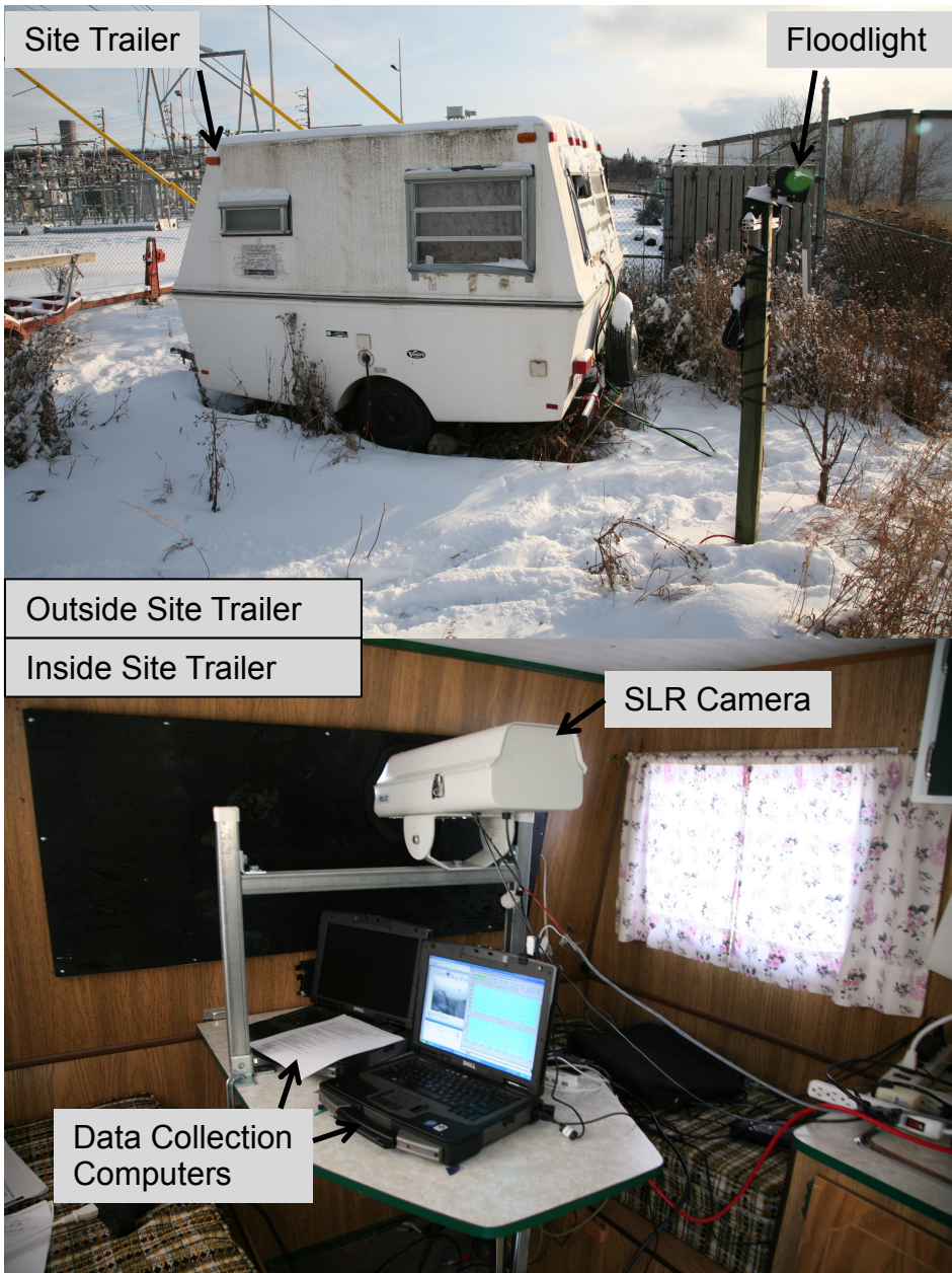
Figure 3-3. Inside and outside picture of site trailer at station 56.8km, housing data collection computers and SLR camera.
