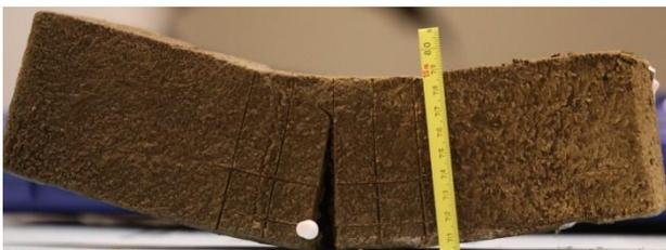
Figure 3. Soil sample after loading.
