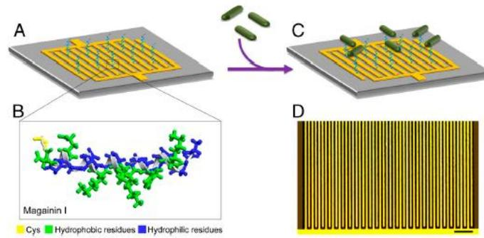
**Figure 4.2** (A) Immobilisation of AMP Magainin on a microelectrode array.(B) Magnified image of Magainin. (C) Detection and binding of bacteria by Magainin. (D) Image of microelectrode array. (Adapted from reference <sup>11</sup>)
