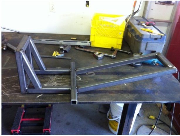
Figure 4.5: (Left) Rear Frame During Construction, (Right) Completed Front and Rear Frames
