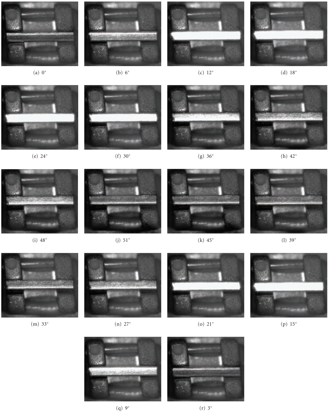
FIGURE 5: Images of the bracket as it is progressively torqued by the archwire. Noted with each image ((a)–(r)) is the angle applied by the single axis torque rig.
