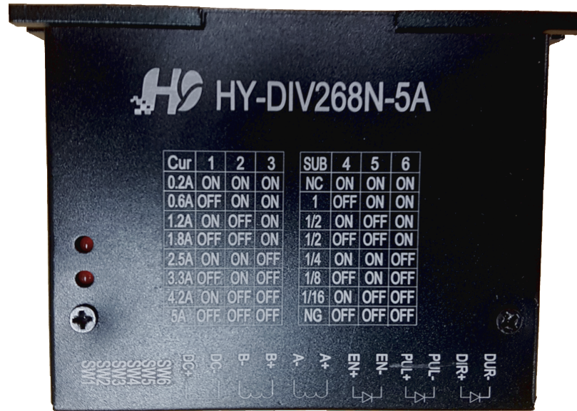
Figure 4.9: Current limiting stepper driver based on the TB6600 chip.
