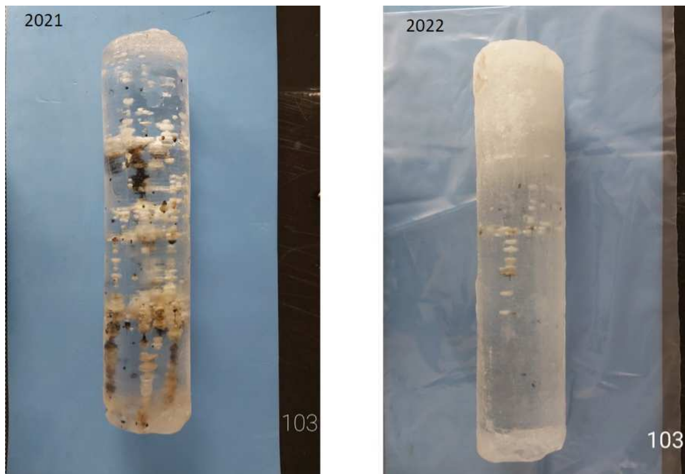
Figure 4-8: Ice cores taken from same location before dredging (2021, on left) and after dredging (2022, on right) demonstrating reduction in bitumen flux post-dredging
