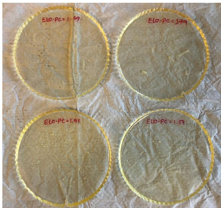
Figure 6.1 Bioresins prepared from epoxidized linseed oil and propyl citrate at 25 °C
