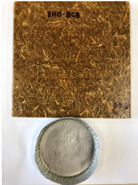
Figure 6.2 A biocomposite and a bioresin mixture samples
