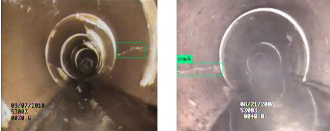
Figure 3. 3: Image on the left shows manually bounding the defect using Microsoft PowerPoint software, image on the right shows YOLOv3 defect detection and bounding
