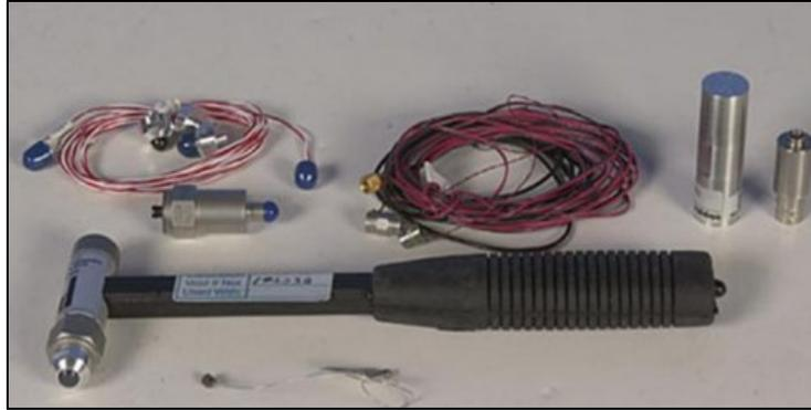
Figure 2. 11: Impulse hammer and accelerometers ([www.used-line.com](http://www.used-line.com)) (Mellett 1995)
