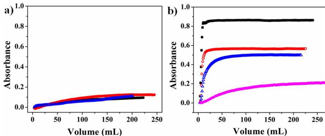
**Figure 5.** The release profiles for the microgel-based etalon devices in (a) pH 6.5 and (b) pH 3.0 solutions. The Au overlayer thicknesses were (■) 50 nm, (●) 200 nm, (△) 500 nm, and (+) 700 nm. In all cases, the total release times were 2 h. Since the flow rates were variable from experiment to experiment, the total volumes are slightly different, but allow for direct comparisons of the data with flow rate irrelevant.
