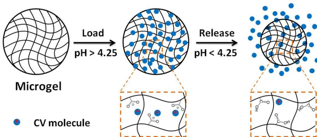
**Figure 2.** The loading and release mechanism of CV molecules into and out of pNIPAm-co-AAc microgels.
