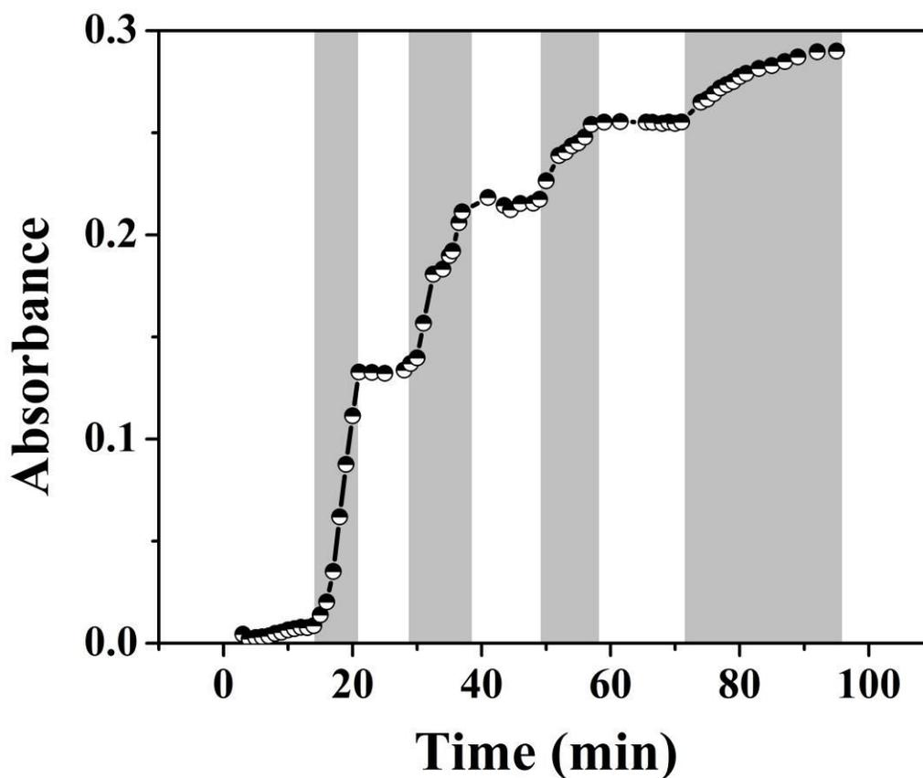
**Figure 7.** pH triggered release profile from an etalon with 500 nm Au overlayer. The dark regions represent where the solution pH was changed to 3.0, while the white regions are where the solution pH was 6.5. As mentioned, the solution pH was varied by adding either HCl or NaOH.
