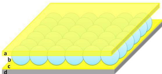
**Figure 1.** Structure of a pNIPAM microgel-based etalon. (a) and (c) are 15 nm Au layers (with 2 nm Cr adhesion layer) sandwiching (b) a microgel layer all on a (d) glass substrate.
