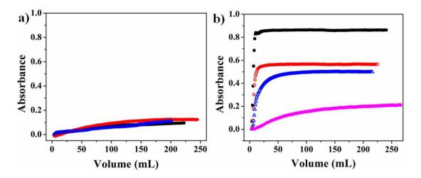
**Figure 5**. The release profiles for the microgel-based etalon devices in (a) pH 6.5 and (b) pH 3.0 solutions. The Au overlayer thicknesses were ( $\blacksquare$ ) 50 nm, ( $\bigcirc$ ) 200 nm, ( $\triangle$ ) 500 nm, and (+) 700 nm. In all cases, the total release times were 2 h. Since the flow rates were variable from experiment to experiment, the total volumes are slightly different, but allow for direct comparisons of the data with flow rate irrelevant.
