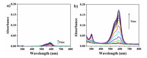
**Figure 4**. Release of CV over time, monitored via UV-Vis spectrophotometer, in (a) pH 6.5 and (b) pH 3.0 solutions. The Au overlayer thickness of this sample was 500 nm. The maximum absorbance is at 590 nm and the absorbance increase with time. The spectra were obtained every 30 sec, and the total release time was 2 h; here we show spectra for the first 10 min of release.
