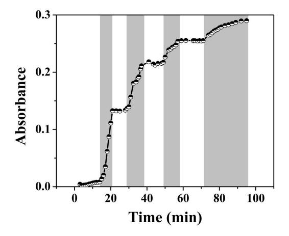
**Figure 7**. pH triggered release profile from an etalon with 500 nm Au overlayer. The dark regions represent where the solution pH was changed to 3.0, while the white regions are where the solution pH was 6.5. As mentioned, the solution pH was varied by adding either HCl or NaOH.
