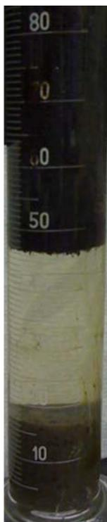
**Figure 3-14:** Image of a cylinder prepared from overflow of secondary cyclone after two months. This photograph is taken after the solids dispersed in water phase completely settled to the bottom of the cylinder.
