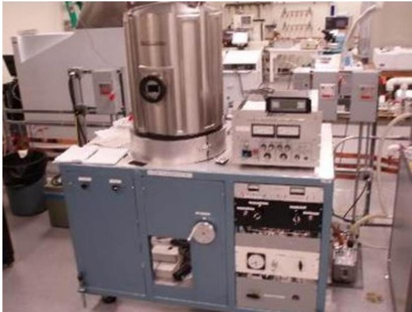
Figure 2.11. Electron beam evaporation system.
