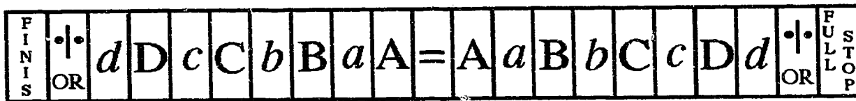
Figure 43. Key layout of Jevons' logical machine
