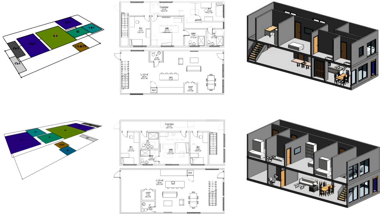
Figure 4-13. Floor plan and 3D view after conversion and modification
