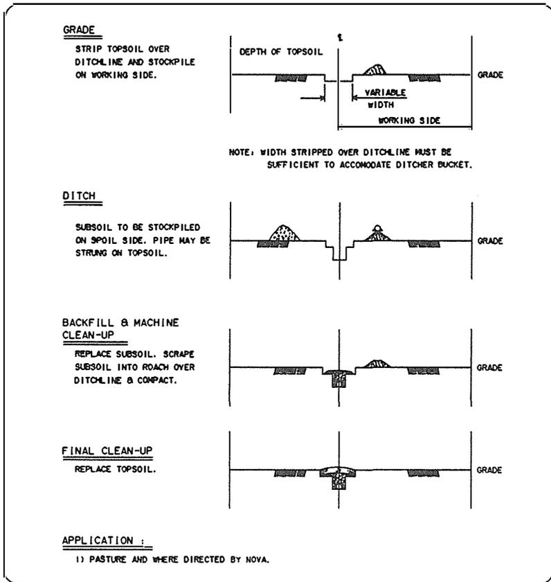
**Figure 3: Ditchline stripping procedure in summer conditions (NOVA 1990)**
