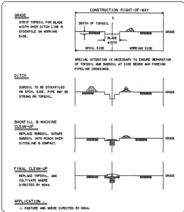
**Figure 4 : Blade width stripping procedure in summer conditions (NOVA 1988)**
