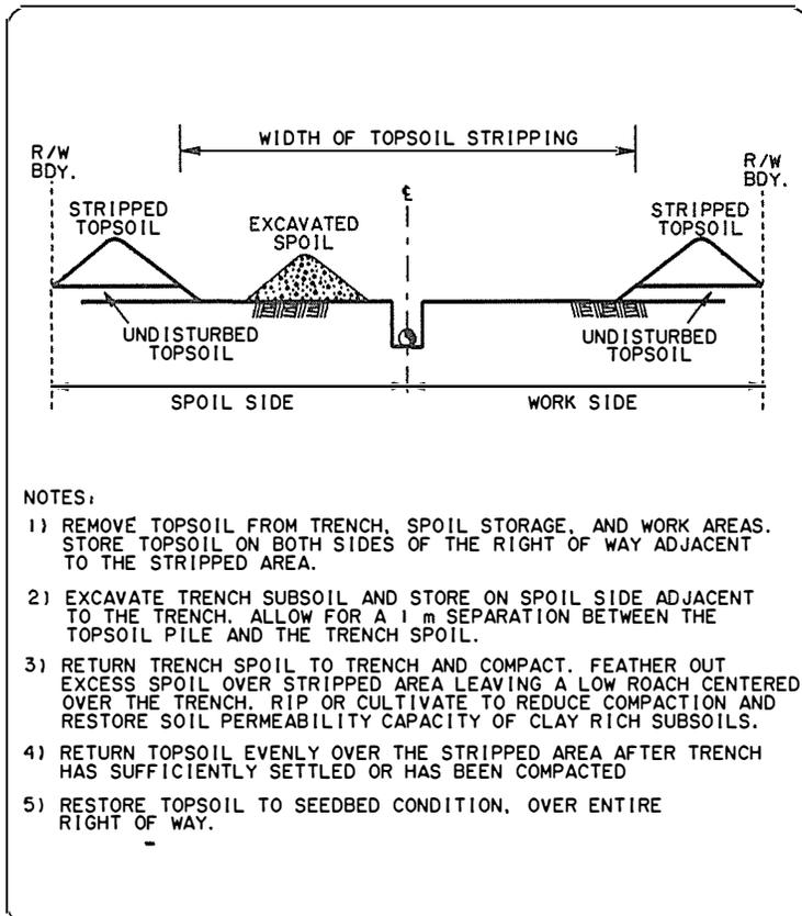
**Figure 6 : Trench, spoil and worksite stripping procedure in summer conditions (Alberta Environment 1985).**
