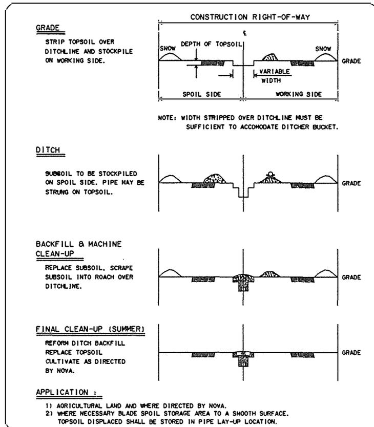
**Figure 7 : Ditchline stripping procedure in winter conditions (NOVA 1988).**
