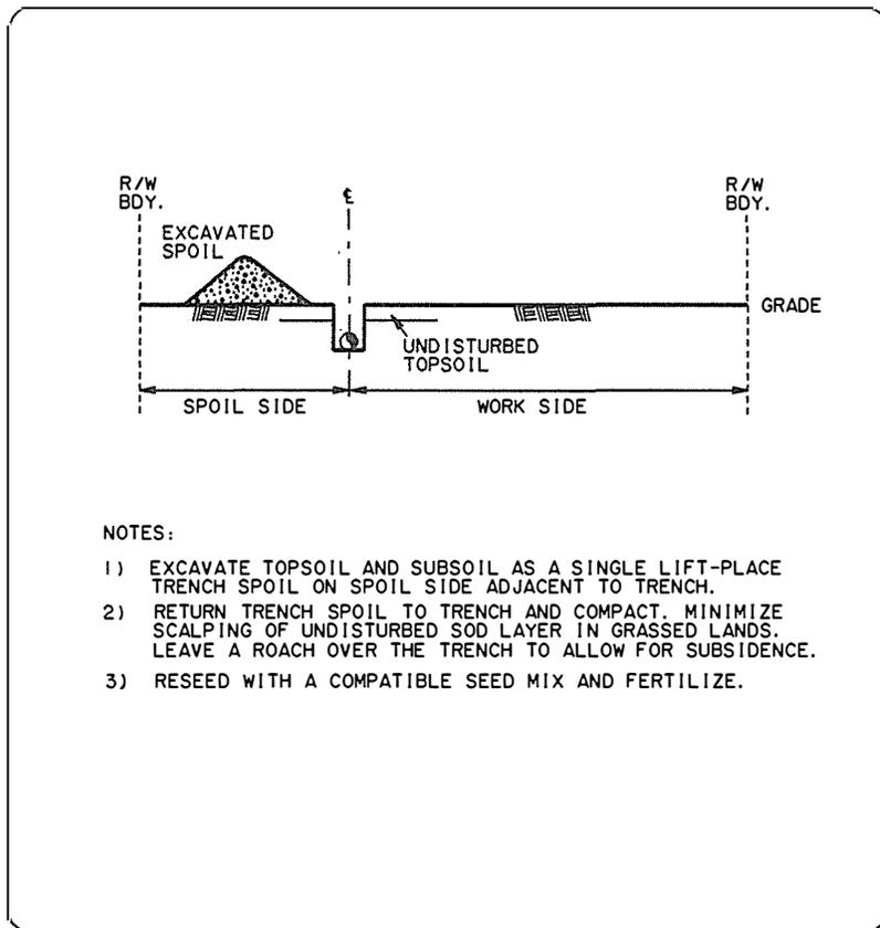
**Figure 2: No topsoil stripping procedure in summer conditions (Alberta Environment 1985)**
