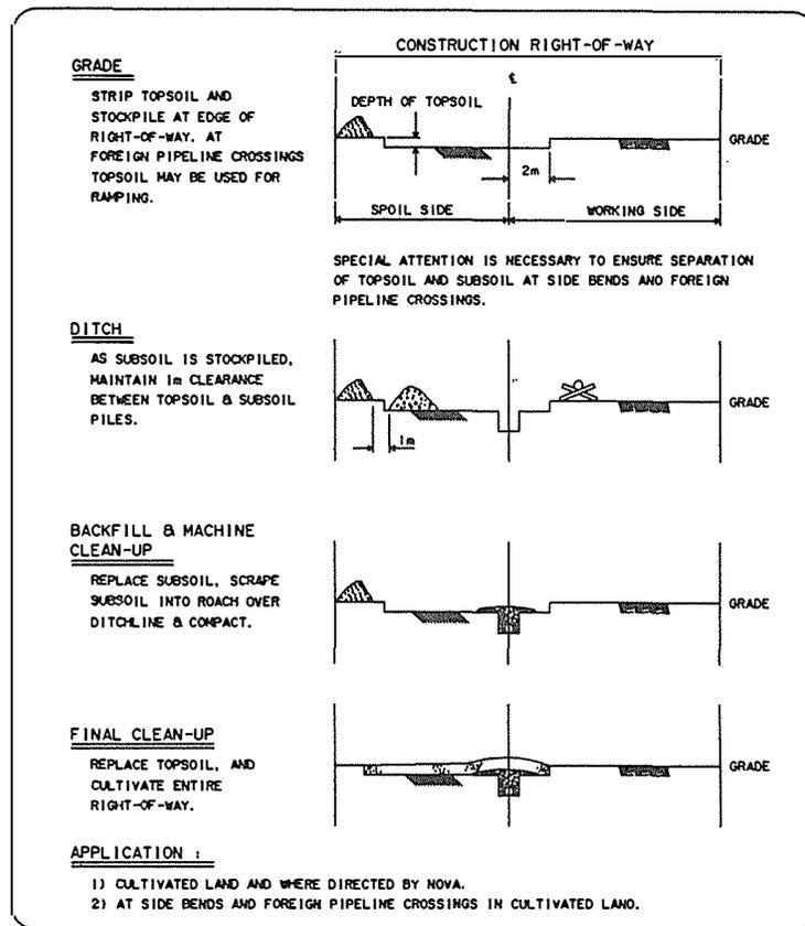
**Figure 5 : Ditchline and spoil side stripping procedure in summer conditions (NOVA 1988)**
