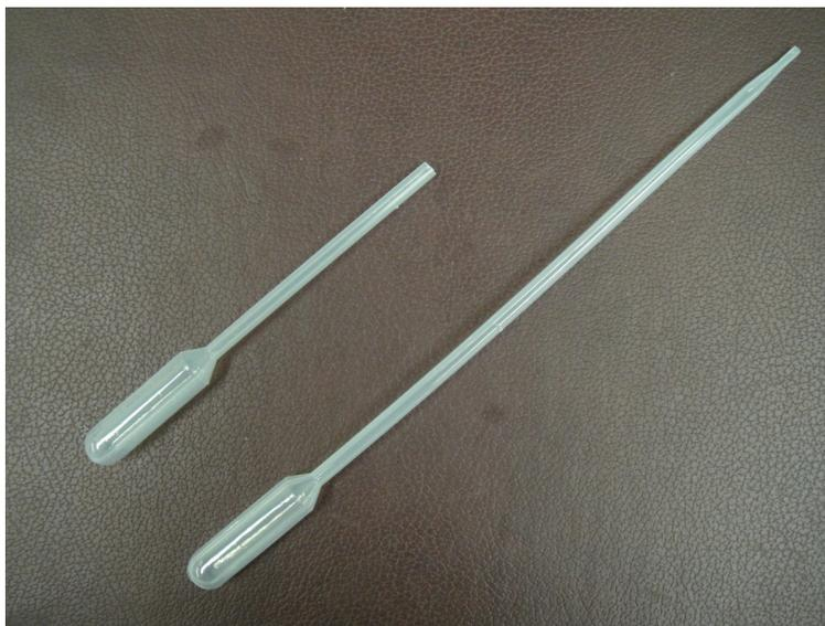
**Figure 3.5. Large-tip opening transfer pipette (13-711-5B Fisher Scientific)**
