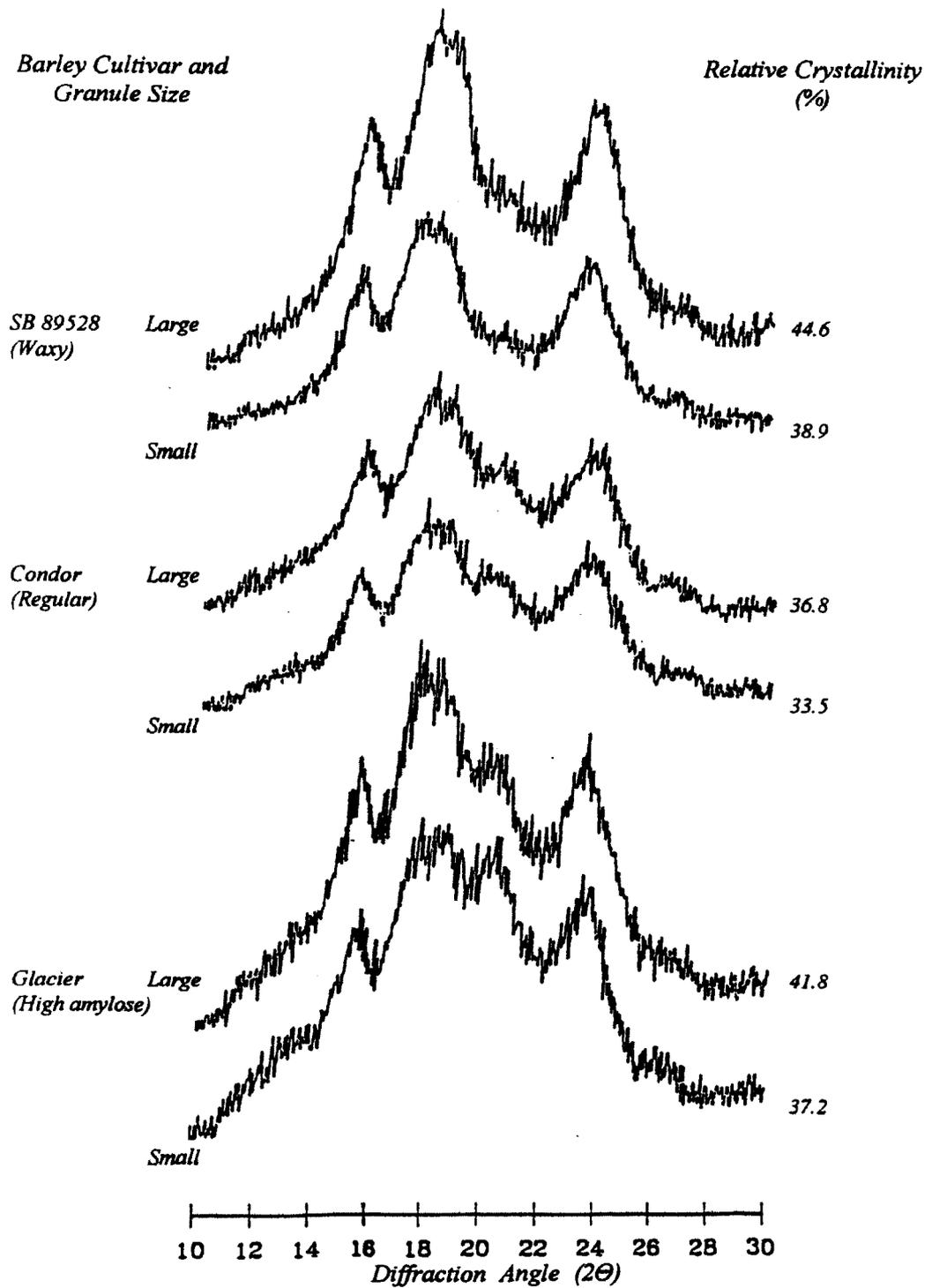
**Figure 2.9** X-ray diffraction patterns and relative crystallinities of regular, waxy and high amylose starches (adapted from Vasanthan and Bhatt, (1996) with minor modification).
