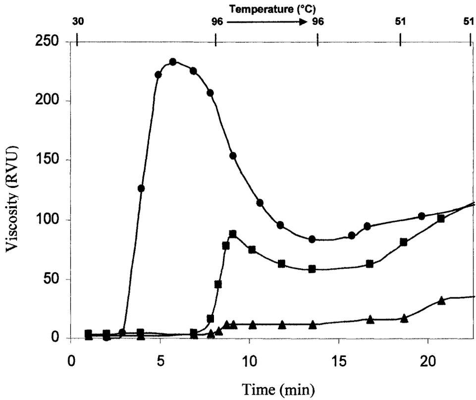
**Figure 2.11** Pasting properties of barley starches measured by a Rapid Visco-Analyzer (adapted from Song and Jane (2000) with minor modification). Waxy (●), regular (■), and high amylose (▲).
