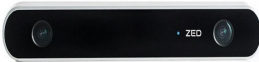
Figure 3-7: ZED stereo camera.
