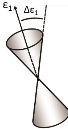
Figure 1.10 Uncertainty cone represents 95% confidence interval of the true dominant fiber orientation \epsilon_1 .
