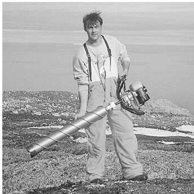
FIG. 6. Tommy Nørnberg standing on top of a peat mound at the Nordvestø peat site (July, 2001), with the assembled corer and one-man (1.6 hp) motor. Although one person can operate the corer, a two-person team is the minimum necessary for safe field operations in Arctic conditions. Having two people also expedites the labeling and packing of the cores.
