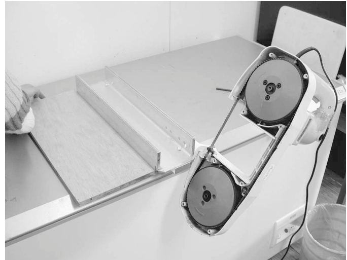
FIG. 4. Horizontally hinged band saw mounted on an aluminum frame, with adjustable backstop for varying the slice thickness. When it is judged safe to do so, and as a necessary requirement for lowest possible cross-contamination of slices, the bottom cover of the band saw is removed during operation to allow quick and easy cleaning between slices so that debris does not accumulate.
