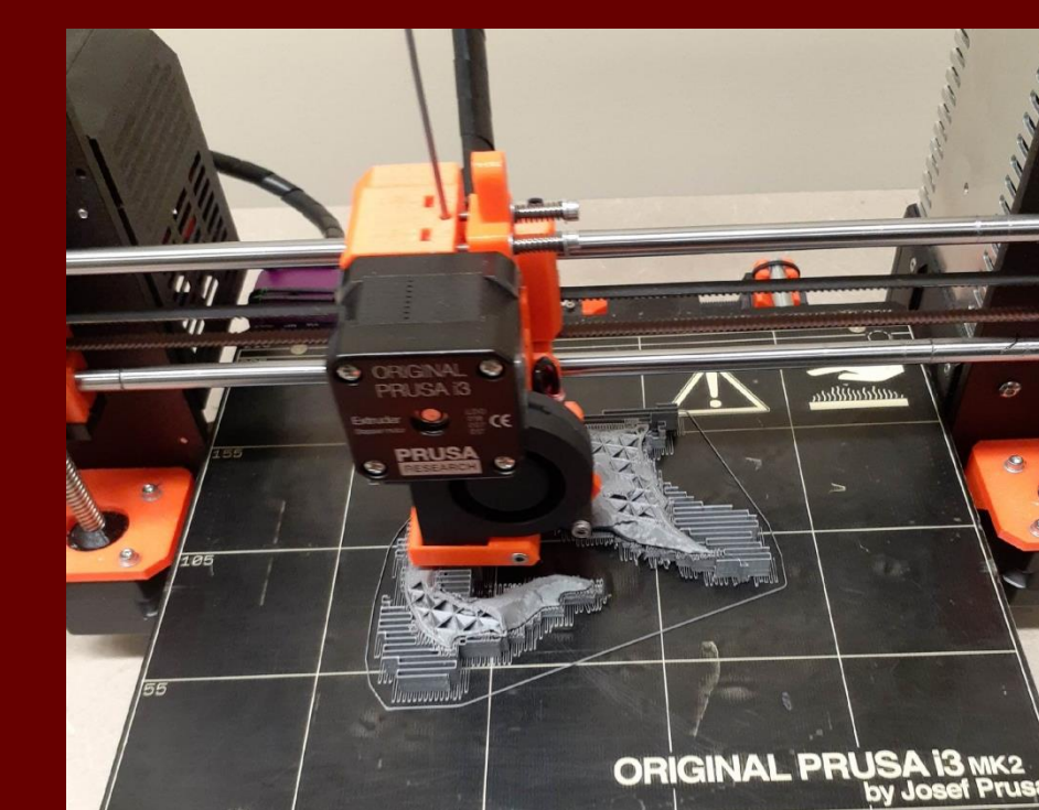
Figure 8: Left Squamosal being Printed on 3D Printer
