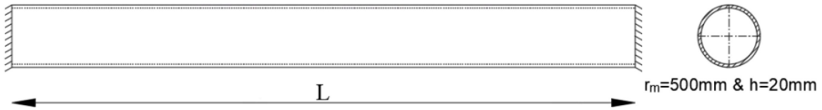
Fig. 5. 4 Geometry of straight pipe
