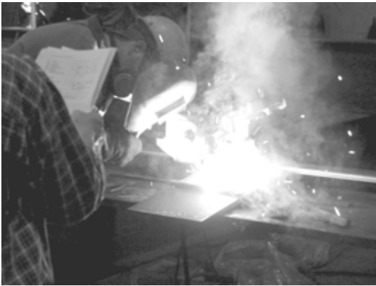
(c) Welding of cruciform specimen
