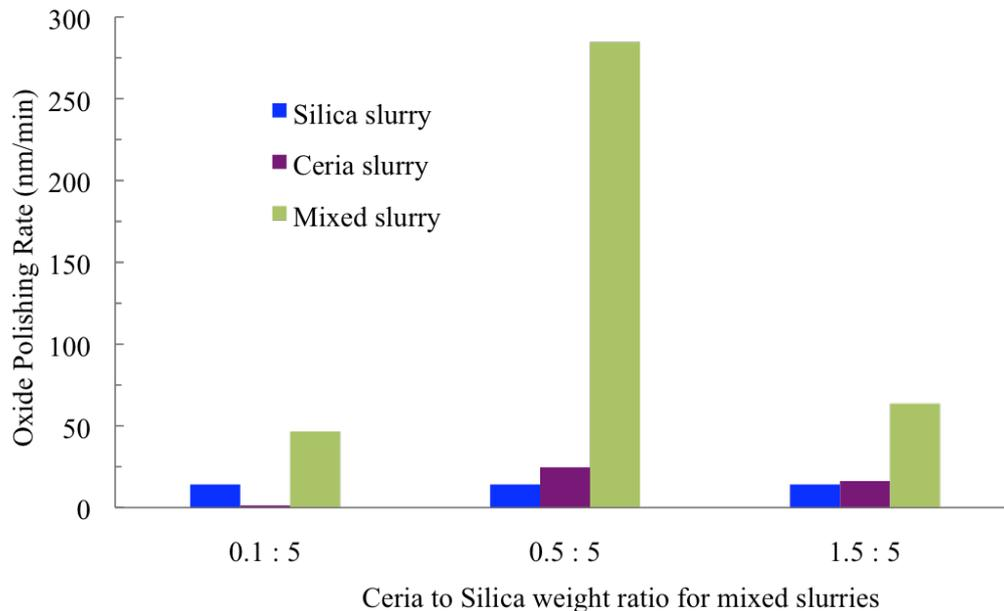
Figure 20 Oxide polishing rates using silica slurry (5 wt%), ceria slurries (0.1 wt%, 0.5 wt% and 1.5 wt% from left to right) and mixed slurries of silica and ceria at pH 4
