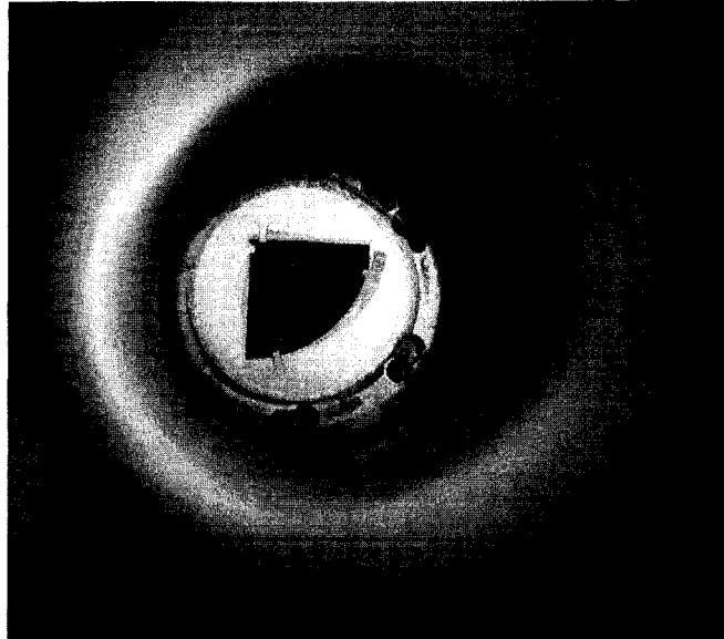
Figure 17: Infrared image of the GaAs substrate in the MBE growth chamber.
