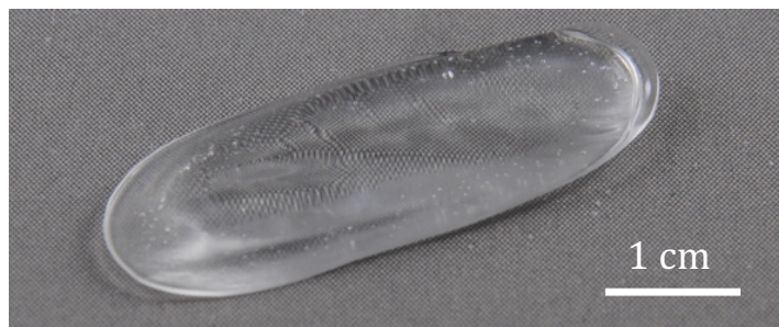
Figure 3-8. Set sodium silicate specimen prepared for in vitro immersion tests. The distortion of the fabric weave, visible through the specimen, indicates the uneven bottom surface and shrinkage void that formed during setting (further detailed in Chapter 4.1.2).
