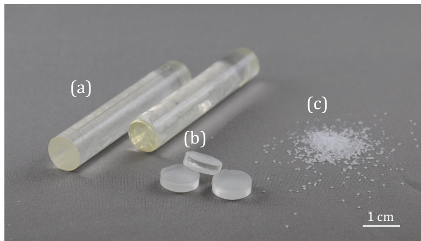
Figure 3-1. 45S5 bioactive glass, as (a) 12 mm diameter rods, (b) discs sectioned from rods, and (c) +355 \mu\text{m} frit.
