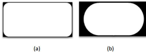
Figure 6.9. Sketch of bubble profiles in a rectangular channel under different flow conditions: (a) Interface shape at Ca < 10^{-3} ; (b) bubble shape at Ca > 10^{-3} in rectangular channel with aspect ratio, width ( w )/depth ( h ) > 1.5 (Völkel, 2009; Hazel and Heil, 2002; Wong et al., 1992).
