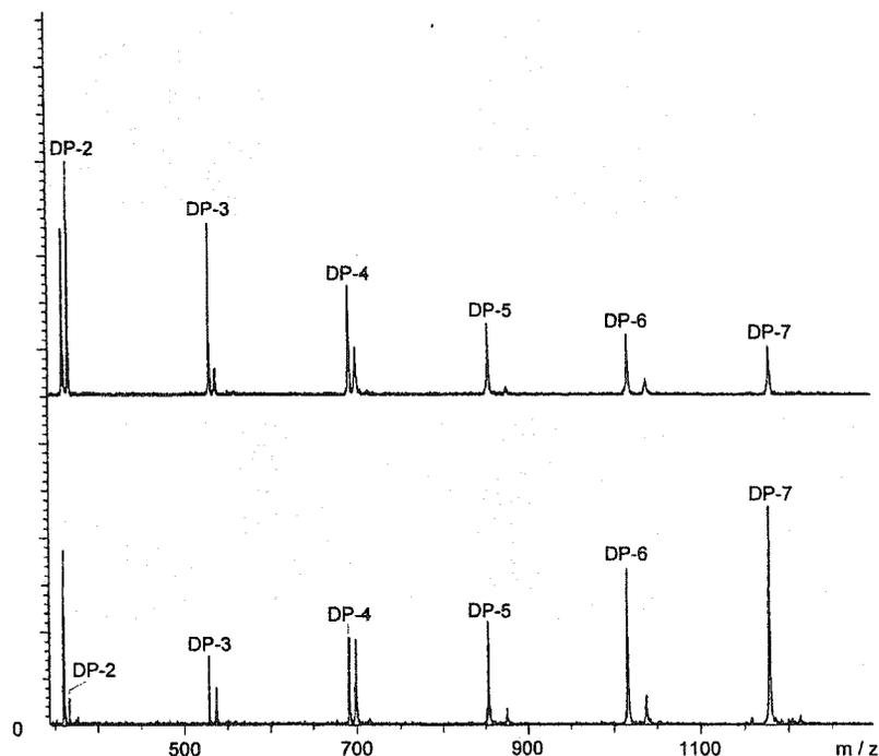
**Figure 3-2.** MALDI-TOF MS positive ion spectra of a mixture of polyol standards (DP-2 through DP-7) dissolved in 0.01 M aqueous NaCl with DHB matrix. Top: equal mass concentrations (0.3 mg/mL); Bottom: equimolar concentrations (0.4 mM). All labeled peaks are  $[M+Na]^+$ . Secondary peaks 8  $m/z$  higher than DP-3 and DP-4 are unidentified. Secondary peaks 22  $m/z$  higher than DP-5 and DP-6 are identified as  $[M + 2Na - H]^+$ .
