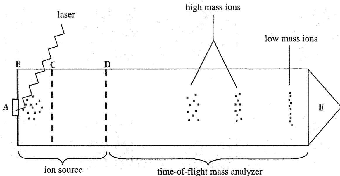
**Figure 1-1.** Schematic diagram of linear matrix-assisted laser desorption/ionization time-of-flight mass spectrometer. A: sample probe tip; B: repeller plate; C: extraction grid; D: acceleration grid; E: detector.
