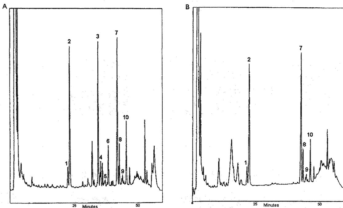
**Figure 2-1.** Typical HPLC chromatograms of ginseng extract monitored at 205 nm where Solvent A is a) phosphate buffer or b) water. 1- Rg<sub>1</sub>, 2-Re, 3-mRb<sub>1</sub>, 4-mRc, 5-mRb<sub>2</sub>, 6-mRd, 7-Rb<sub>1</sub>, 8-Rc, 9-Rb<sub>2</sub>, 10-Rd.
