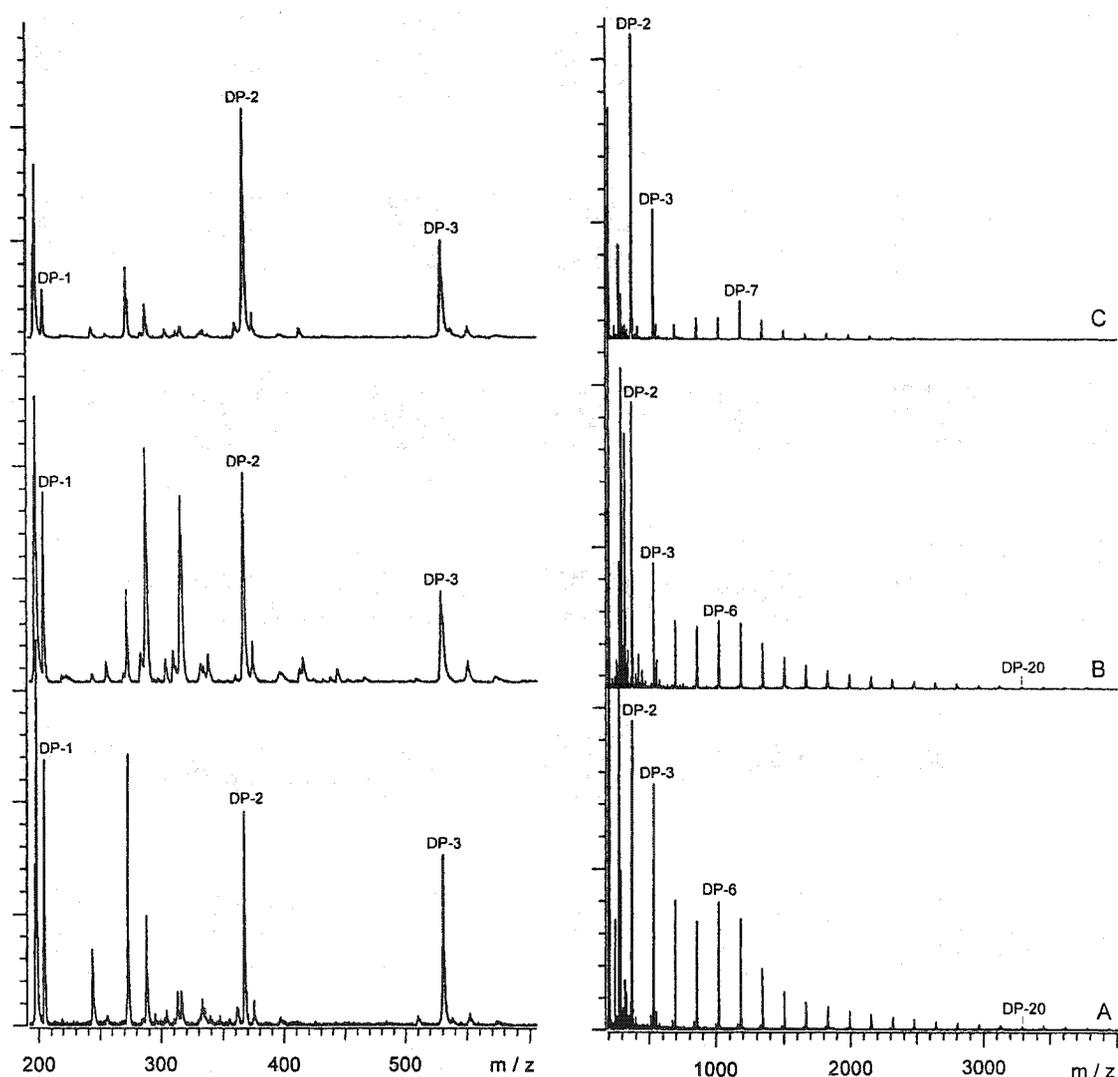
**Figure 3-4.** MALDI-TOF MS positive ion spectra of a) low, b) medium, and c) high maltitol syrups. Left: expansion of mass region  $m/z$  200-500. All sample peaks are  $[M+Na]^+$  ions. Extraneous peaks at  $m/z < 500$  are from the DHB matrix.
