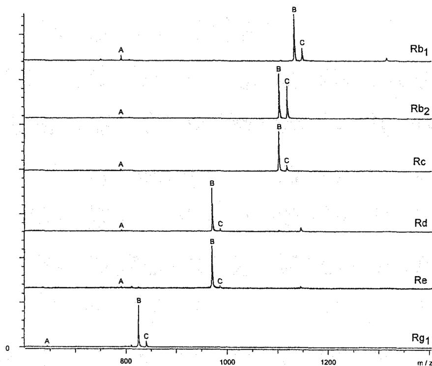
**Figure 2-2.** MALDI-TOF MS spectra in positive ion mode of ginsenoside standards Rb<sub>1</sub>, Rb<sub>2</sub>, Rc, Rd, Re, and Rg<sub>1</sub> dissolved at 1 mg/mL in 50% aqueous methanol. A:  $[M - (\text{sugar at C20}) + H]^+$ ; B:  $[M+Na]^+$ ; C:  $[M+K]^+$ .
