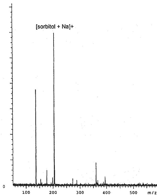
**Figure 3-3.** MALDI-TOF MS positive ion spectrum of 0.5 µg of sorbitol in water with DHB matrix.
