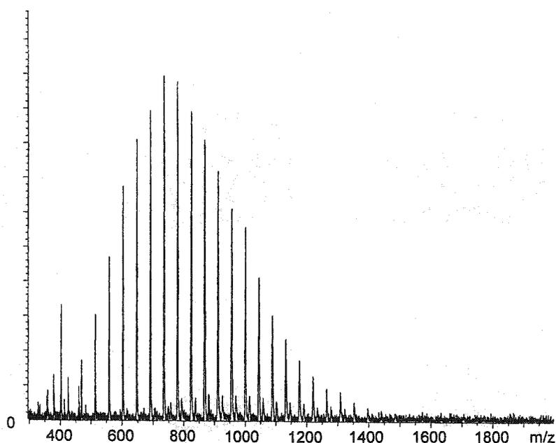
**Figure 7-1.** MALDI-TOF MS spectrum of Brij™ 76 (polyoxyethylene (10) stearyl ether) in 0.01M NaCl with THAP matrix.
