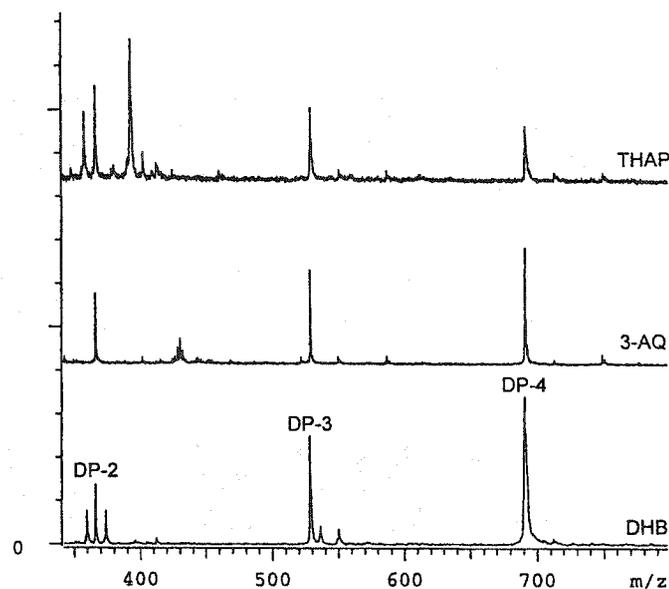
**Figure 3-1.** MALDI-TOF MS positive ion spectra of polyol standards with three matrices. A mixture of maltitol (DP-2), maltotriitol (DP-3), and maltotetraitol (DP-4) at equimolar concentrations (1.0 mM) was prepared in 0.01 M aqueous NaCl.
