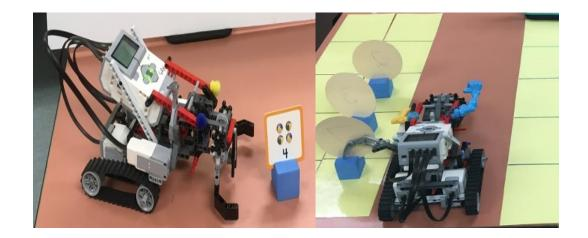
*Figure 2*. Lego Mindstorms robot with a gripper to grasp objects on top of blocks (left), and with a pointer to point at the objects (right).
