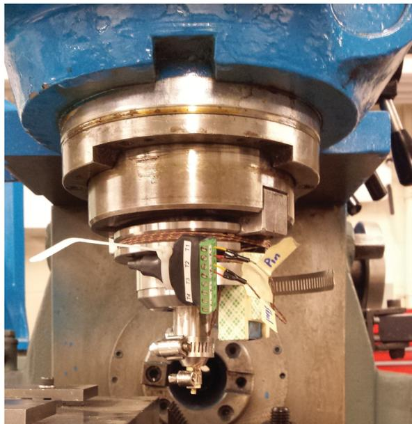
Figure 3.3: Experimental set-up to measure FSW tool pin and shoulder temperature
