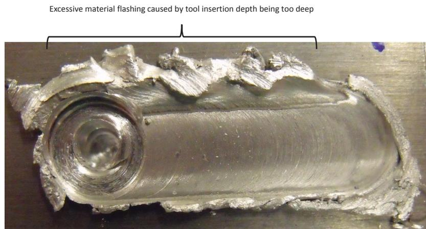
Figure 4.8: Tool D weld defect - excessive material flashing caused by large tool insertion depth
