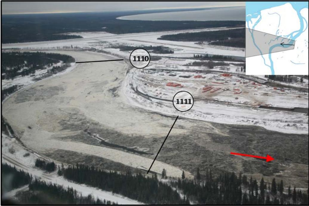
Figure 2.5 Image showing the juxtaposed ice cover formation in the East Channel during 2008 freeze-up.
