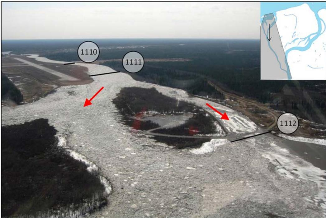
Figure 2.17 Image of the ice jam in the West Channel delta on 4-May-09.
