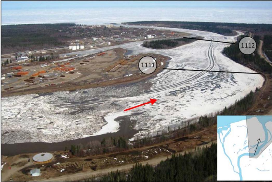
Figure 2.16 Image of ice jam in the East Channel on 4-May-09.
