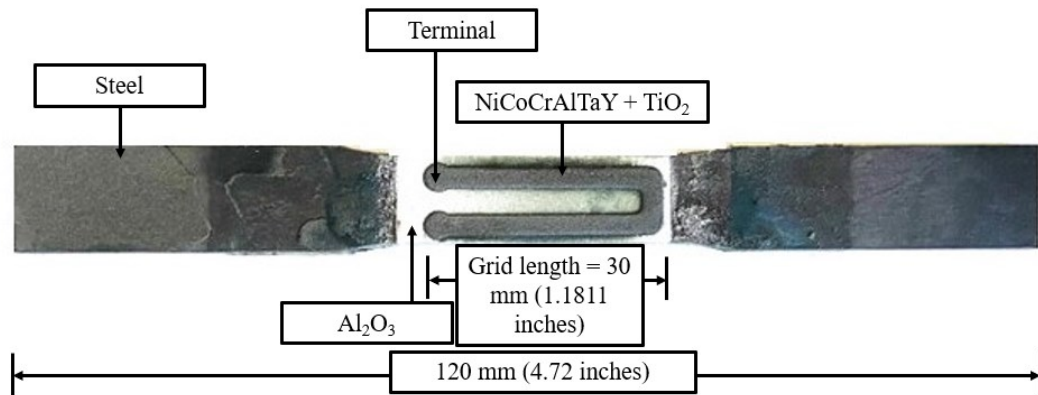
Figure 2-6 Steel sample after deposition of alumina and nickel alloy
