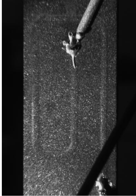
Figure 2-15 Image from fast imaging cameras used to measure 2D strain for carbon fiber reinforced polymer (CFRP)
