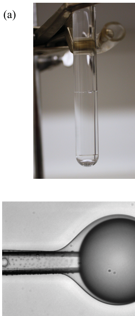
Figure 5-3: Upon contacting the oil phase ( n -hexadecane with 5 wt% AOT) with the brine (water with 3.5 wt% NaCl), a third phase — a bicontinuous (BC) liquid — appeared spontaneously. (a) The so-called Winsor III mixture in a test tube, with the oil phase at the top, the aqueous phase in the middle, and the BC phase at the bottom (this BC phase was more dense than the brine); (b) the BC phase was seen to spontaneously engulf an oil droplet that was held at the pipette tip; the oil droplet was roughly 60 \mu\text{m} in diameter. The surrounding liquid was brine.
