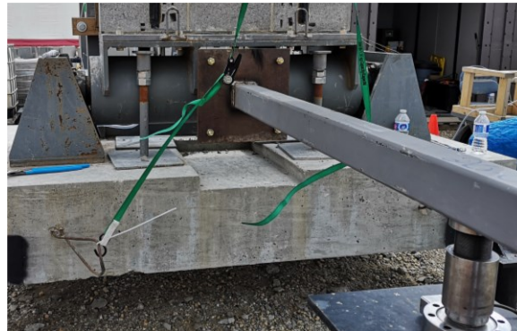
Figure 4.3 – Rotational base stiffness simulation
