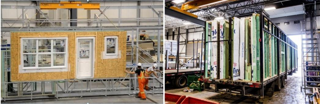
Figure 4.10: Loading trailer (courtesy of ACQBUILT, Inc.)
