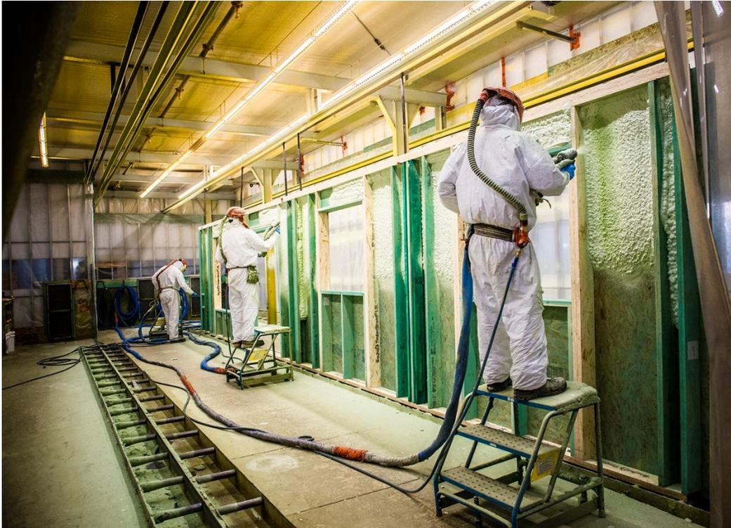
**Figure 4.6: Exterior insulation booth (courtesy of ACQBUILT, Inc.)**
