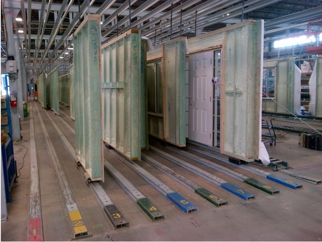
Figure 4.9: Wall magazine line (courtesy of ACQBUILT, Inc.)
