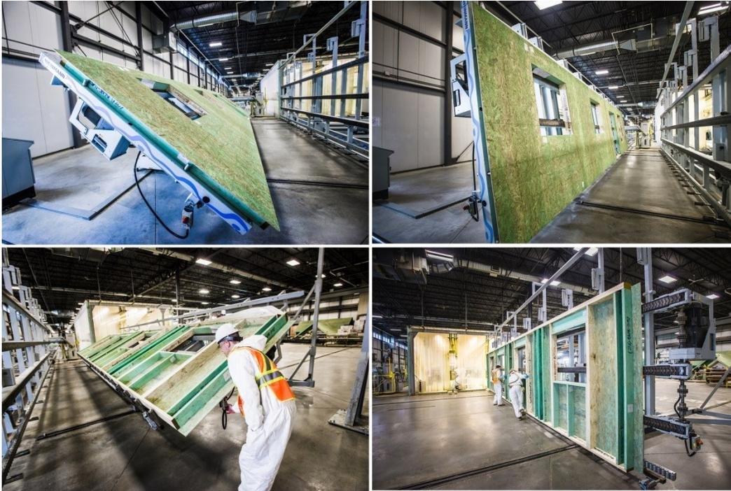
**Figure 4.5: Butterfly table station (courtesy of ACQBUILT, Inc.)**
