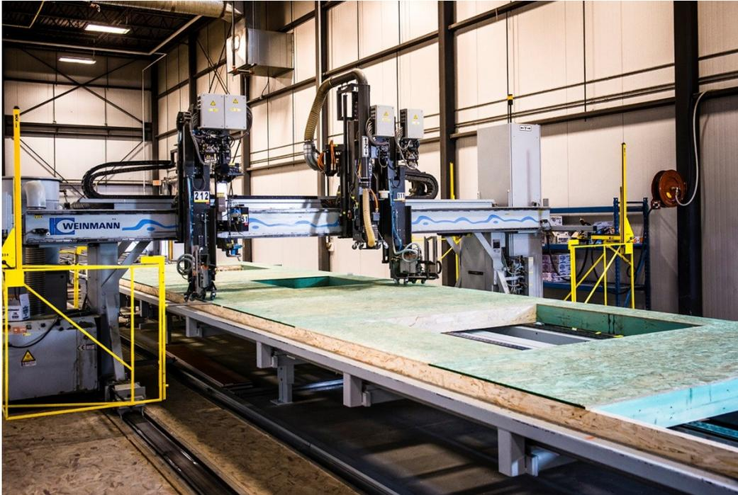
**Figure 4.4: Multi-function bridge (courtesy of ACQBUILT, Inc.)**
