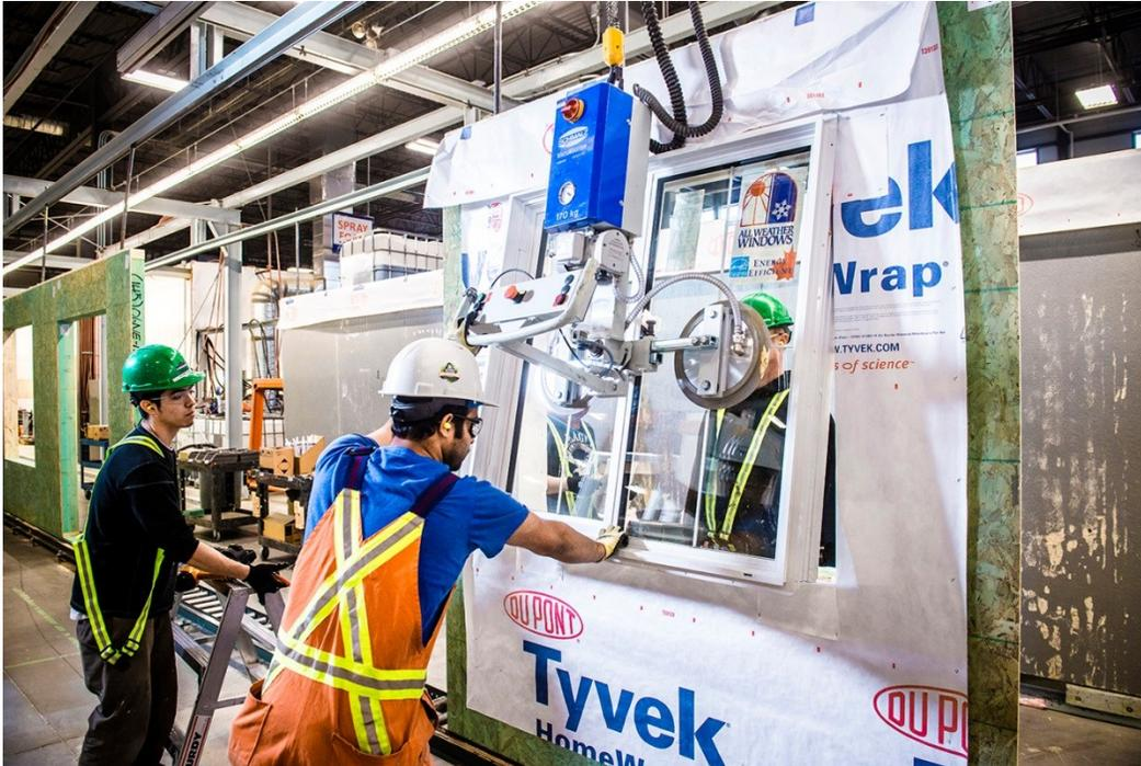
Figure 4.7: Window/door installation line (courtesy of ACQBUILT, Inc.)
