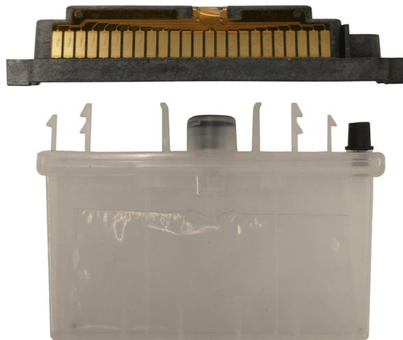
(b) DMC-11610 cartridge printhead (above) and reservoir (below).
