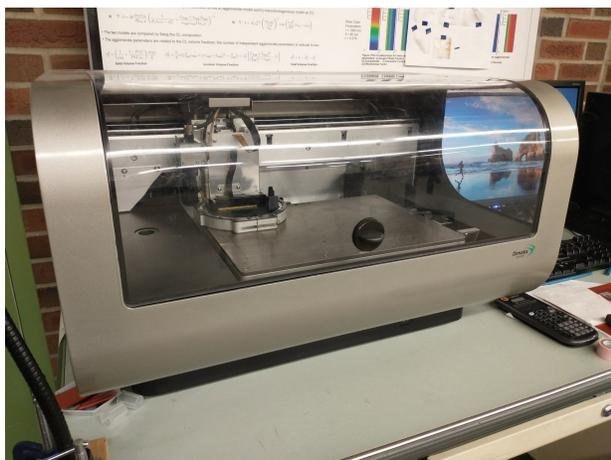
(a) Fujifilm Dimatix DMP-2831 drop-on-demand inkjet printer.
