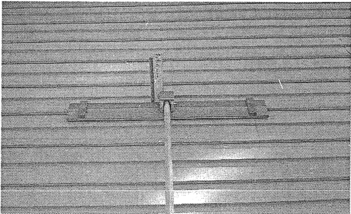
Figure 3.8 Laser plumb measuring aid.
