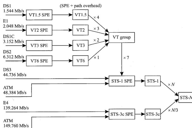
Figure C.5: Mapping of virtual tributaries into an STS-1 SPE (copied from [8]).
