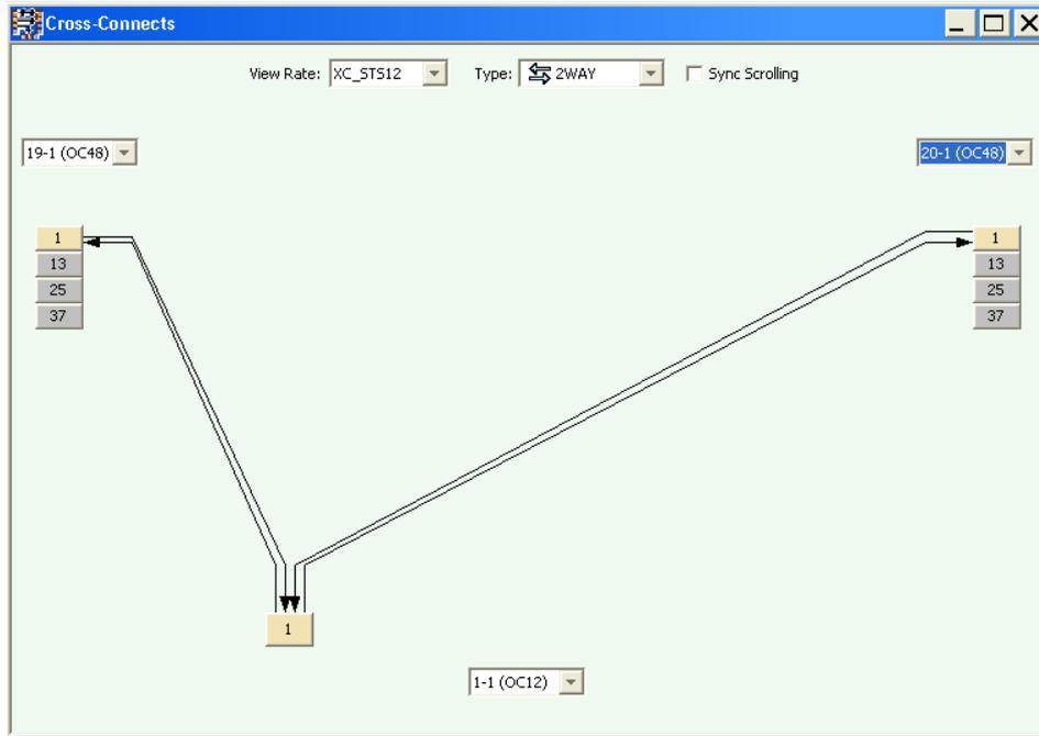
Figure B.4: Rack #2 - UPSR configuration: Cross-connection between the OC-12 and OC-48 circuits.
