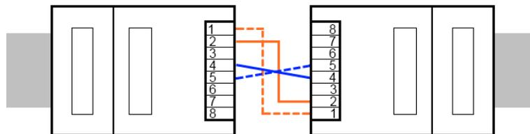
Figure D.1: Pin-out for the straight T1 cable.
