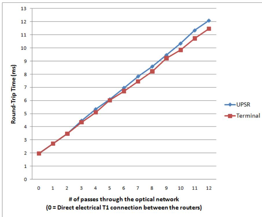
Figure 3.1: Round-trip times in the UPSR and terminal network configurations.
