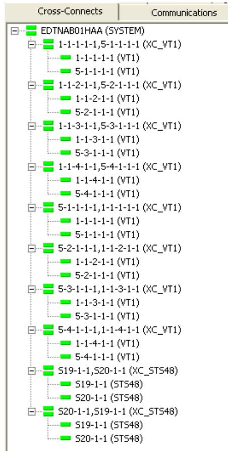
Figure B.3: Rack #1 - UPSR configuration: Cross-connects view when the DS1 signal is sent through the network four times.
