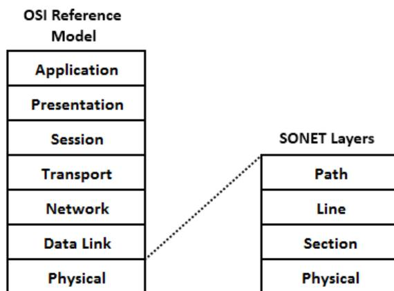
Figure C.3: The seven layers of the ISO OSI reference model and the four SONET layers.
