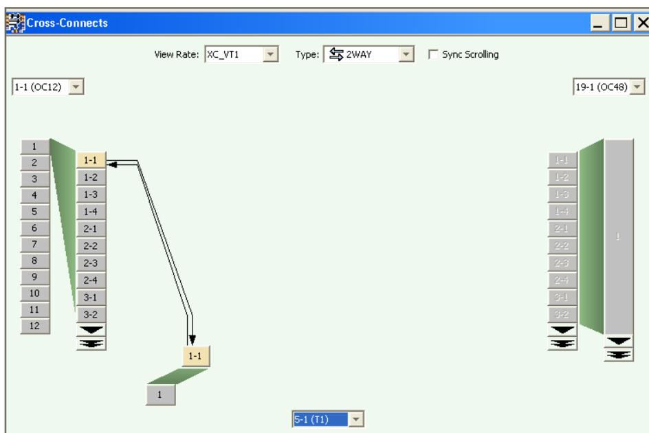
Figure B.5: NE1 and NE2 - Terminal configuration: Cross-connect between a T1 and an OC-12 circuit.
