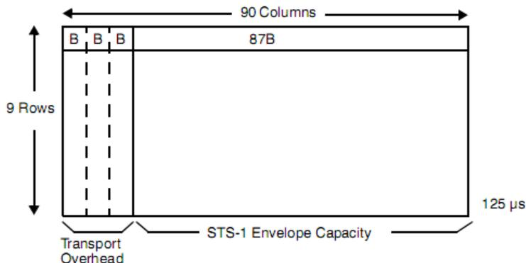
Figure C.4: Illustration of a SONET STS-1 frame (copied from [9]).
