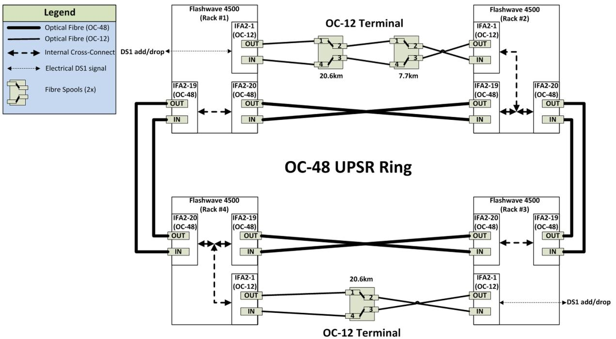
Figure 2.4: Physical layout of the optical part of the network in the UPSR configuration.
