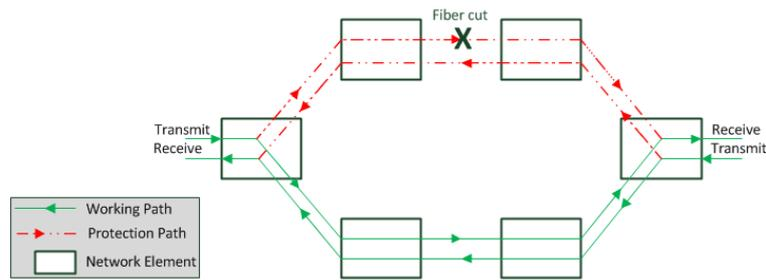
Figure C.7: UPSR with one fibre cut. Notice that only the affected fibre is switched out, the other direction of traffic is unchanged (adapted from [4]).
