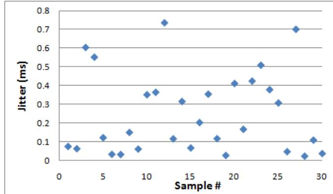
Figure 3.4: Jitter in the configuration shown in Figure 2.2 for a sending rate of 1.48 Mbps.
