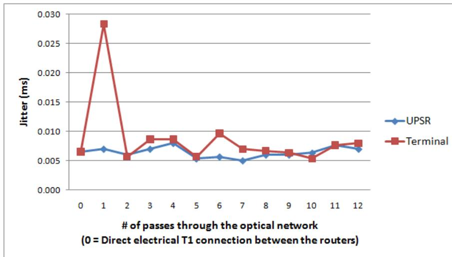
Figure 3.3: Jitter in the UPSR and terminal configurations for a sending rate of 1 Mbps.
