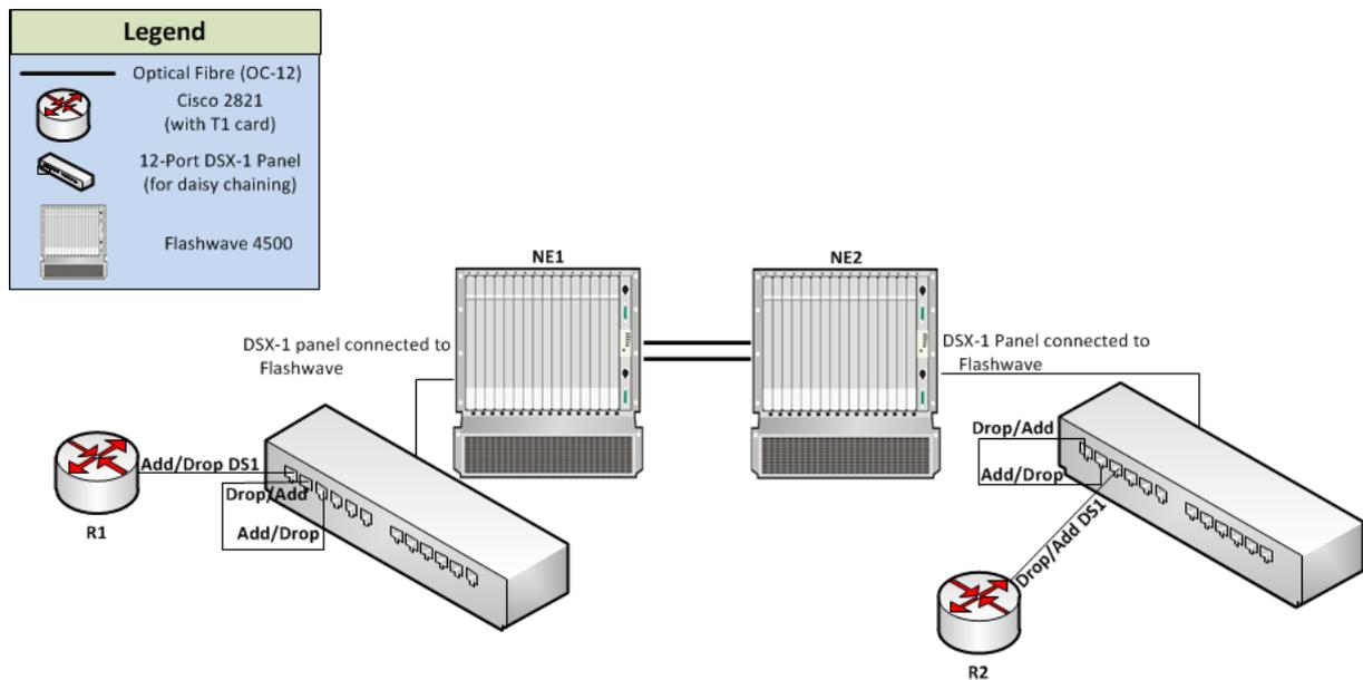
Figure 2.1: Looping of a DS1 signal in order to increase the number of o-e-o conversions as well as the total network length (DSX-1 panel icons are enlarged to show the looping).
