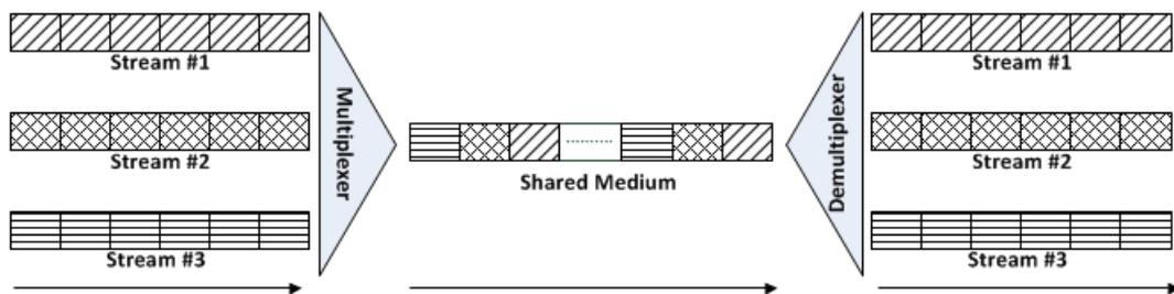
Figure C.1: Example TDM system where three data streams are multiplexed, transported and then demultiplexed.
