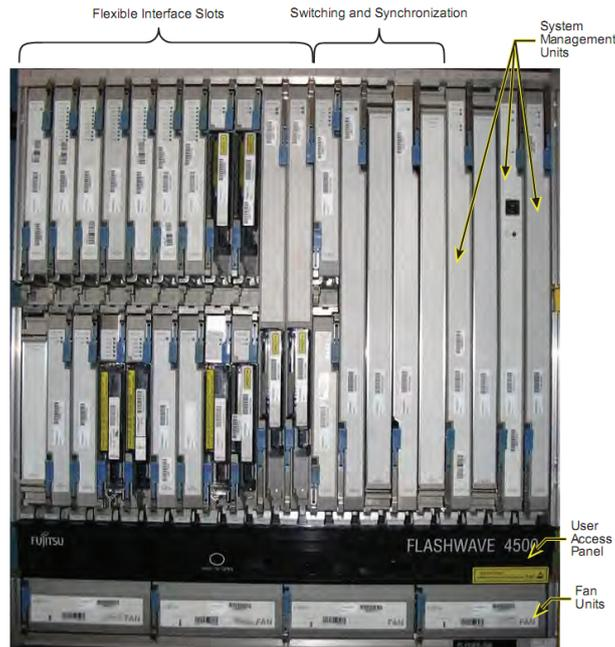
Figure A.1: Front view of the Flashwave 4500 (from [4]).
