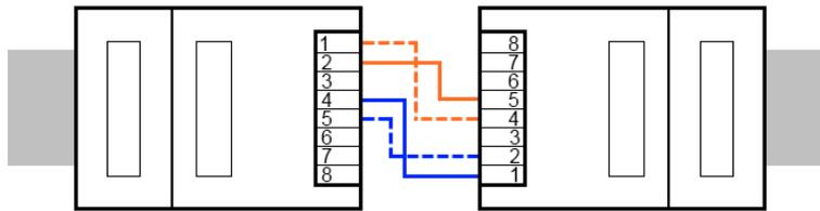
Figure D.2: Pin-out for the crossover T1 cable.
