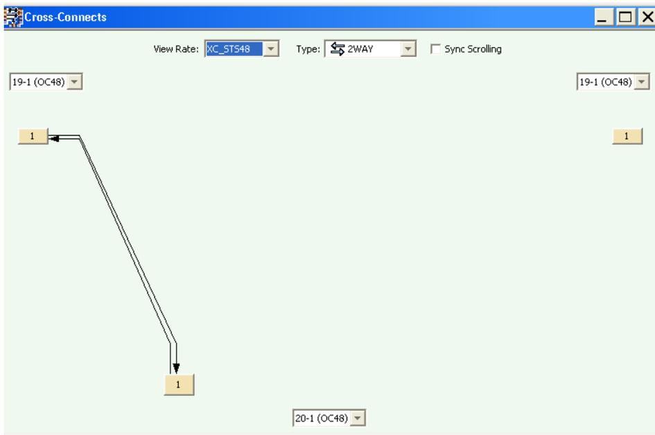
Figure B.2: Rack #1 - UPSR configuration: OC-48 pass-through cross-connect
