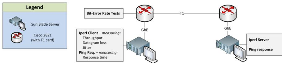
Figure 2.2: Direct electrical T1 connection between two routers.
