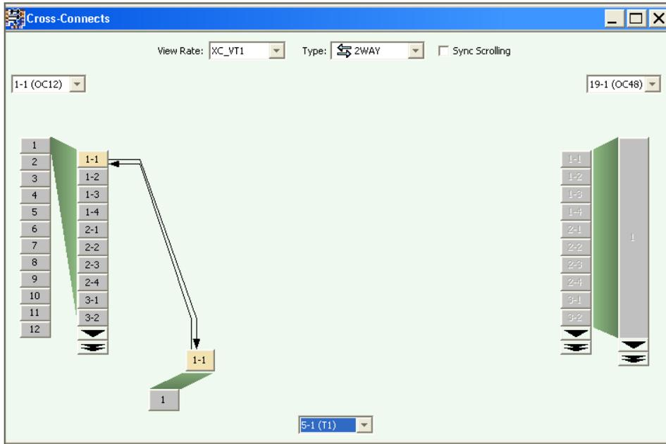
Figure B.1: Rack #1 - UPSR configuration: Cross-connect between a T1 and an OC-12 circuit.
