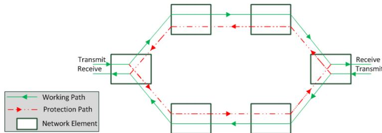
Figure C.6: UPSR during normal operation (adapted from [4]).
