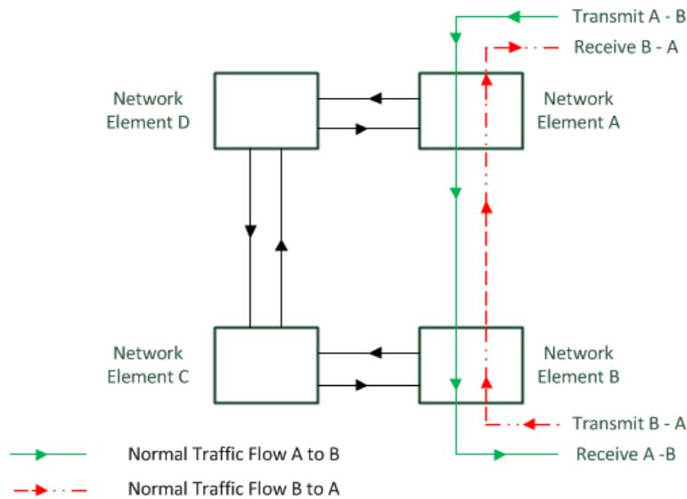
Figure C.8: A 2F-BLSR under normal working conditions (adapted from [4]). The traffic is carried in the working timeslots over both fibres in the span between network elements A and B.
