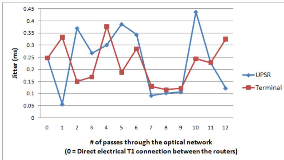
Figure 3.5: Jitter in the UPSR and terminal configurations for a sending rate of 1.48 Mbps.
