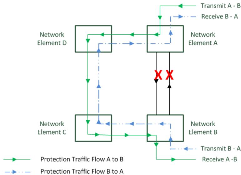
Figure C.9: A 2F-BLSR after fibre cuts in the A to B span (adapted from [4]). The traffic is carried in the protection timeslots over the fibres in the new path between A and B in both directions.
