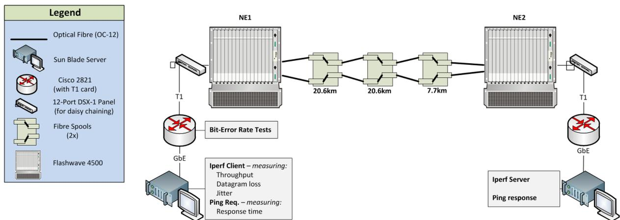
Figure 2.5: Terminal network configuration.
